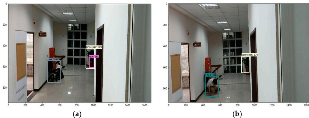
**Figure 20.** (a) The person is unable to be detected; (b) The person is detected as another object.
