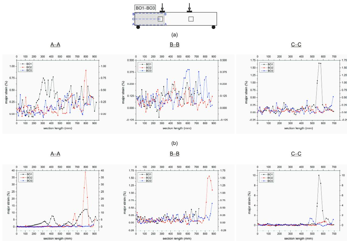
**Figure 12.** Major strains of concrete beam (BO1) and hybrid fibre concrete beams (BO2, BO3) with openings: (a) at service load, and (b) at maximum load.
