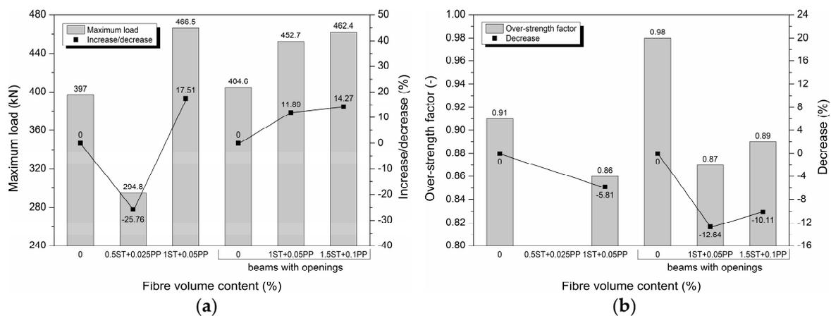
Figure 8. Comparison of beam (a) maximum load and (b) over-strength factor.
