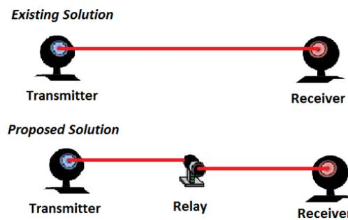
Figure 1. Synoptic diagram of the proposed blind detection free-space optical (FSO) system.
