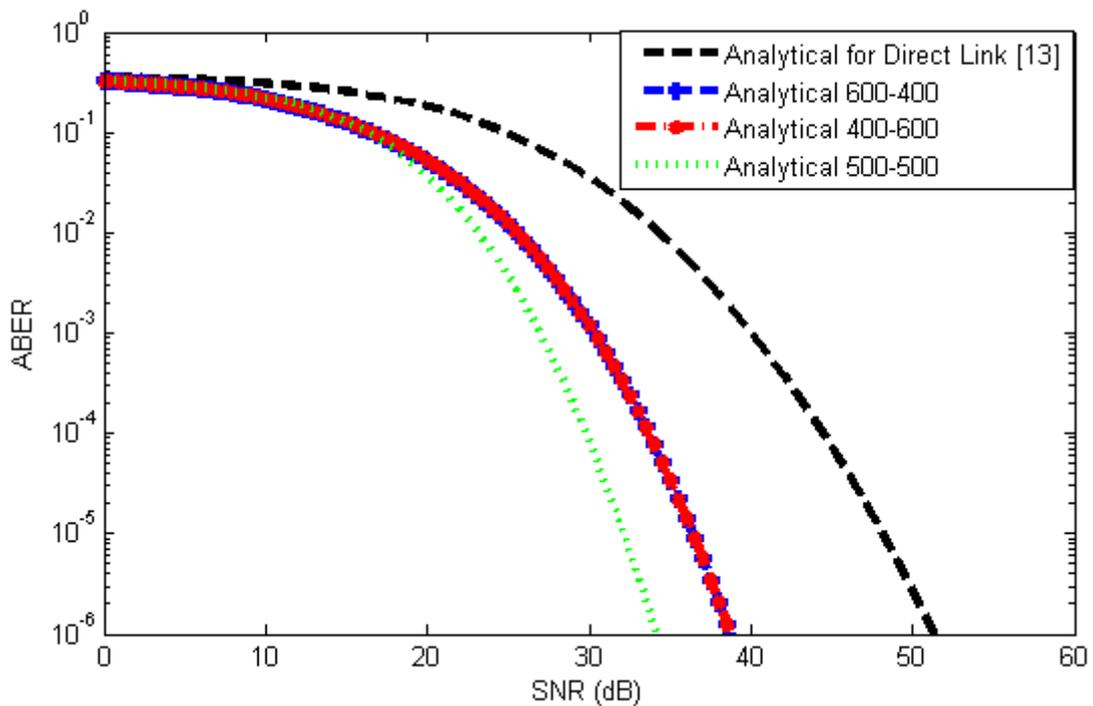
**Figure 5.** ABER performance for the direct link and a single relay with different locations, over moderate turbulence.
