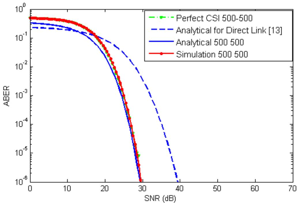
Figure 2. ABER performance for the direct link and a single equidistant relay, over weak turbulence.
