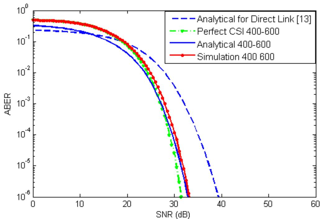
Figure 3. ABER performance for the direct link and a single relay after 400 m from the source, over weak turbulence.
