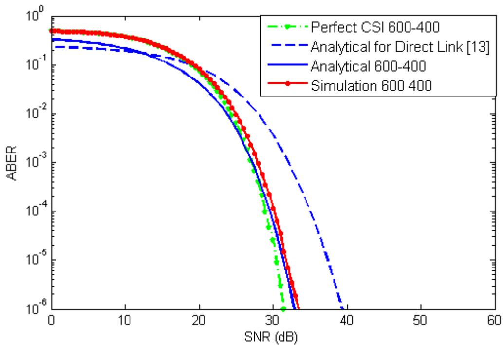
**Figure 4.** ABER performance for the direct link and a single relay after 600 m from the source, over weak turbulence.
