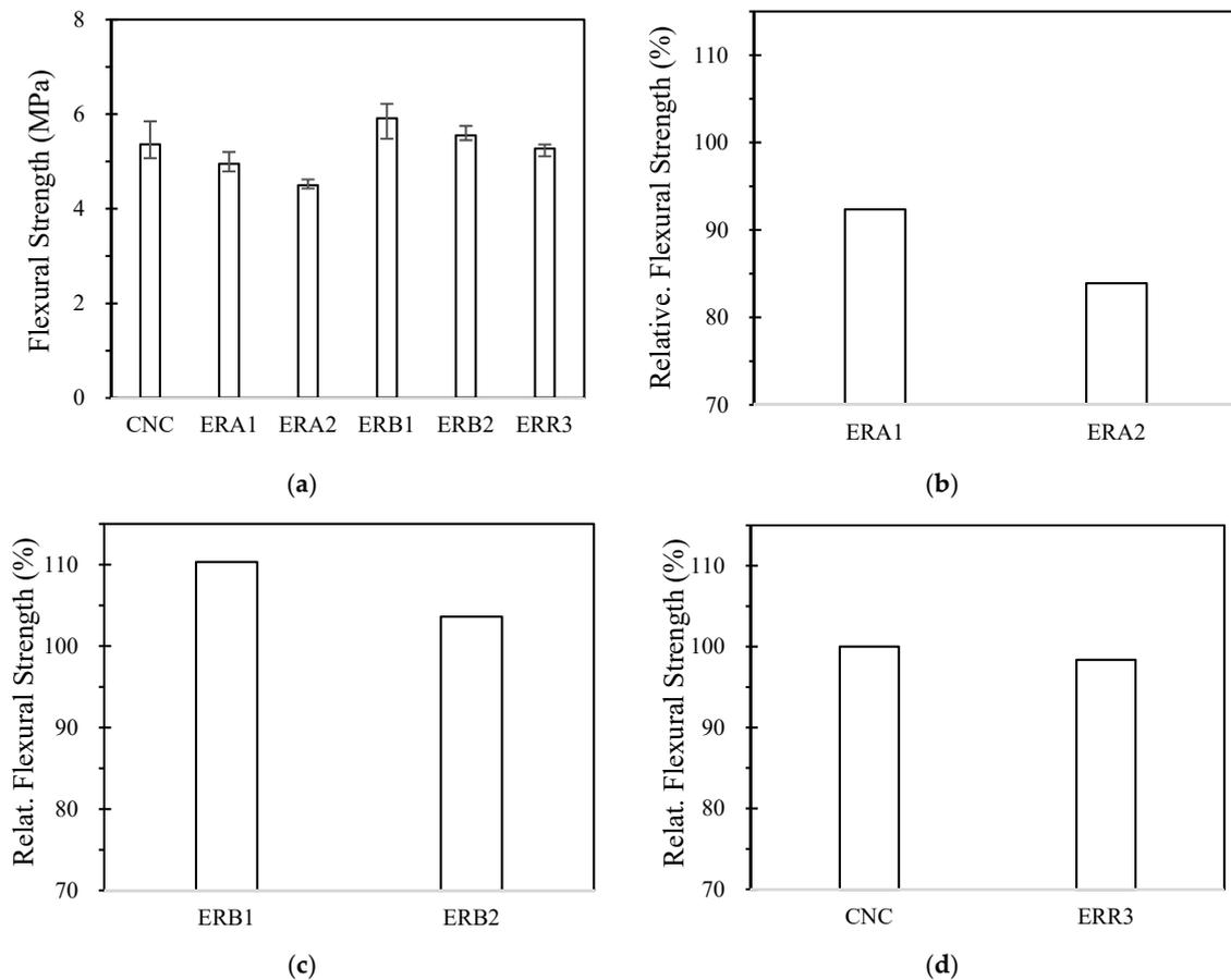
**Figure 8.** Flexural strength results of concrete samples (a) strength, (b) relative value of ERA series, (c) relative value of ERB series, and (d) relative value of ERR mix.
