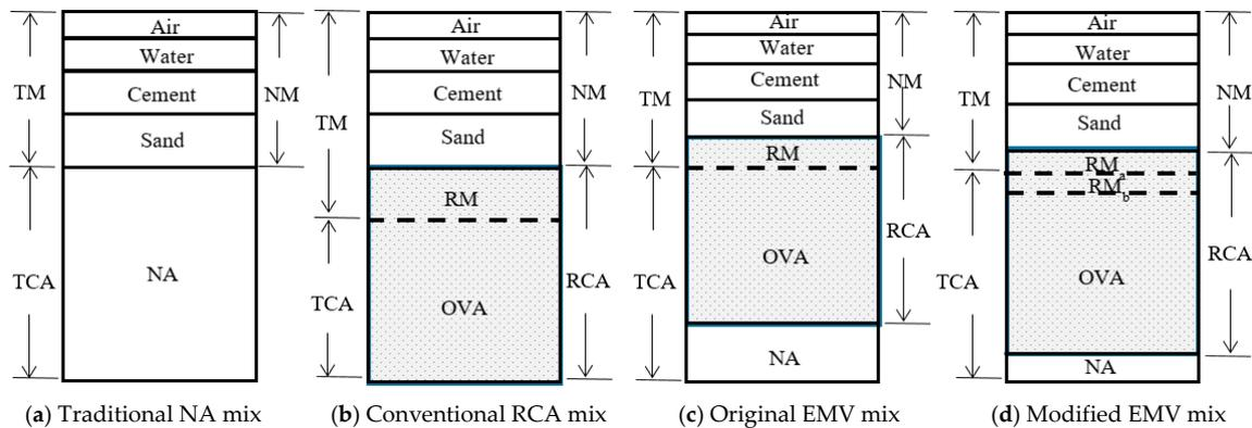
**Figure 1.** Schematic diagrams of different mix designs; TM: Total Mortar; TCA: Total Coarse Aggregate; NA: Natural Aggregate; NM: New Mortar; RM: Residual Mortar; OVA: Original Virgin Aggregate; RCA: Recycled Concrete Aggregate.
