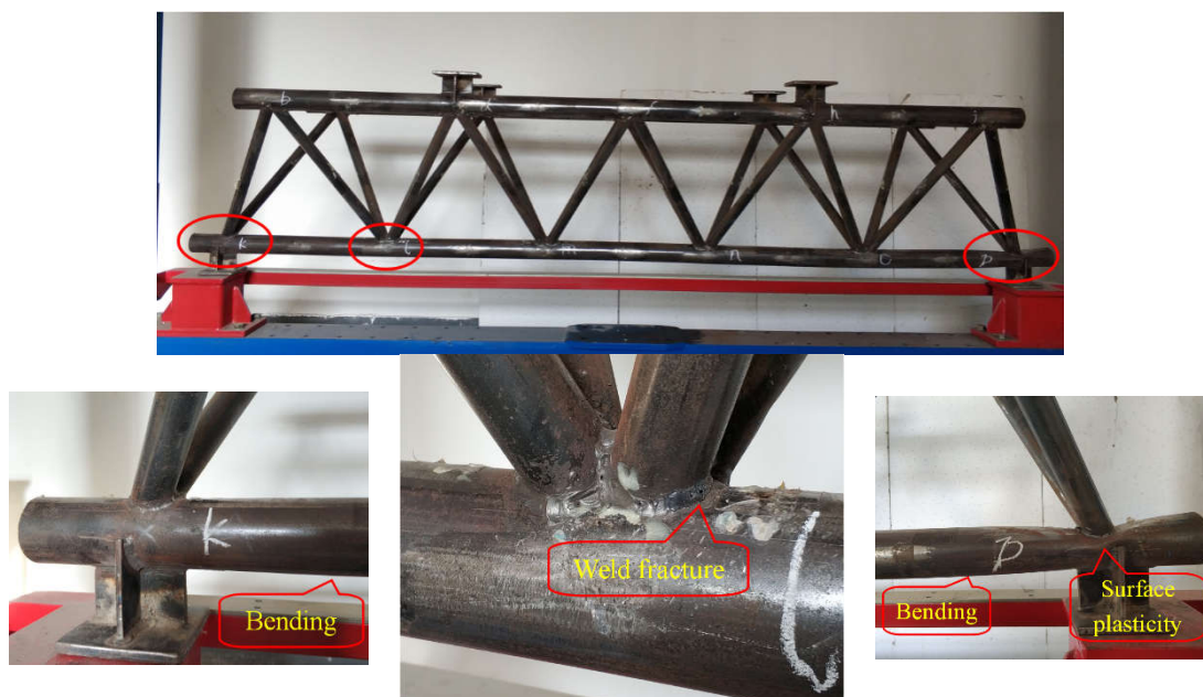
Figure 6. Failure modes of specimen T-HN.
