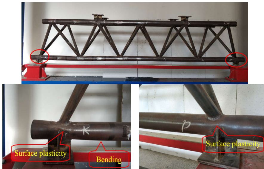
Figure 5. Failure modes of specimen T-HW.
