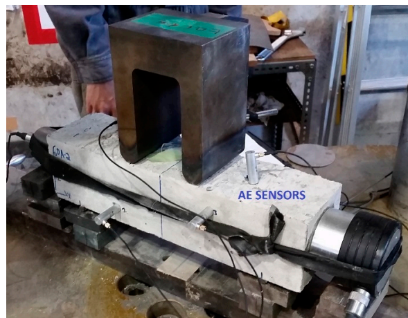
Figure 6. Acoustic emission and four-point bending test setup.
