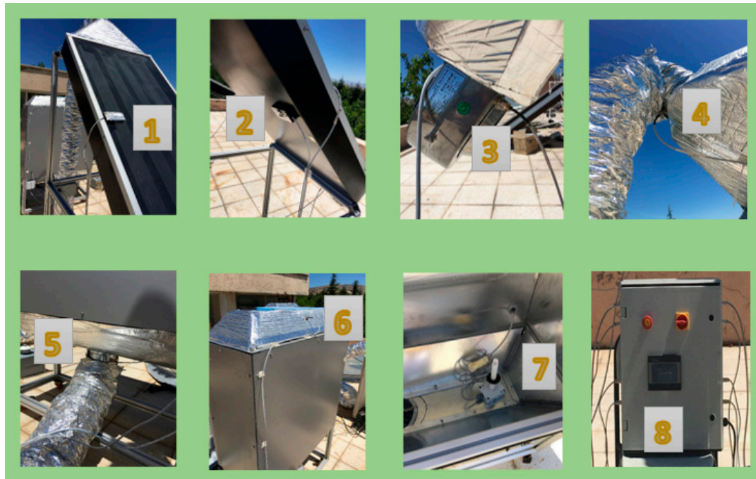
Figure 2. The measuring points: (1) Panel glass temperature; (2) panel floor temperature; (3) panel inlet temperature; (4) panel outlet temperature; (5) drying cabinet inlet temperature; (6) drying cabinet outlet temperature; (7) drying cabinet temperature; (8) measurement monitoring screen.
