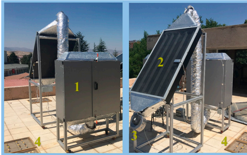
Figure 1. Experimental set-up: (1) drying cabinet; (2) solar collector; (3) circulation fan; (4) pear drying under the sun.
