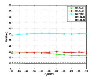
**Figure 8.** RMSE versus transmit power  $P_0$  when  $\sigma = 4$  dB,  $\alpha_f = 0.01$  dB/m (f = 34 kHz), N = 10, and  $\rho = 0.8$ .
