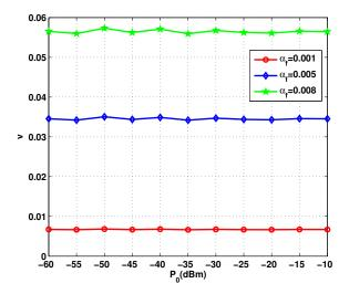
**Figure 3.**  $\nu = \frac{\alpha_f \ln 10}{10\gamma\beta_i}\eta$  versus the transmit power  $P_0$  in Equation (18) for several  $\alpha_f$ .
