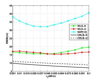
**Figure 7.** RMSE versus absorption coefficient  $\alpha_f$  when  $\sigma = 4$  dB, N = 10, and  $\rho = 0.8$ .
