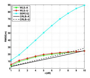
**Figure 4.** Root mean square error (RMSE) versus the  $\sigma$  when N = 10,  $\alpha_f = 0.001$  dB/m (f = 9 kHz), and  $\rho = 0.8$ .
