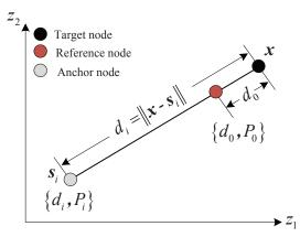
Figure 1. The *i*-th sensoring link in the underwater acoustic wireless sensor network (UWSN) model.
