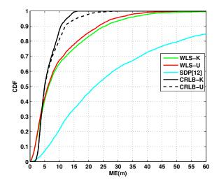
**Figure 6.** Cumulative density function (CDF) versus mean error (ME) when  $\sigma = 4$  dB,  $\alpha_f = 0.1$  dB/m (f = 454 kHz), N = 10, and  $\rho = 0.8$ .
