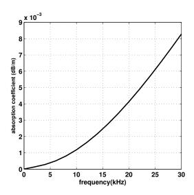
**Figure 2.** Absorption coefficient,  $\alpha_f$ , versus frequency.
