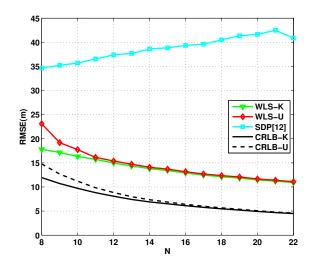
**Figure 5.** RMSE versus the anchor node number *N* when  $\sigma = 4$  dB,  $\alpha_f = 0.01$  dB/m (f = 34 kHz), and  $\rho = 0.8$ .
