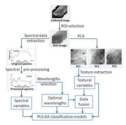
Figure 1. Main steps involved in the measurement and classification of WHC of fresh chicken breast.
