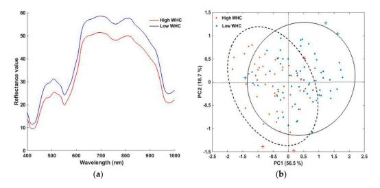
**Figure 2.** Spectral features of chicken breast fillets: (**a**) mean original spectra of high-WHC and low-WHC samples, (**b**) scatter plot of PCA with confidence ellipses (95% confidence level) for samples of high WHC and low WHC.
