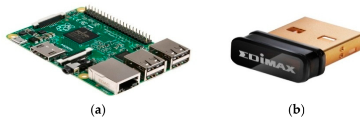
Figure 2. (a) Raspberry Pi model 2B; (b) Edimax Wi-Fi dongle.
