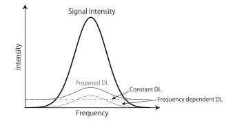
Figure 2. Proposed diagonal loading (DL) technique.
