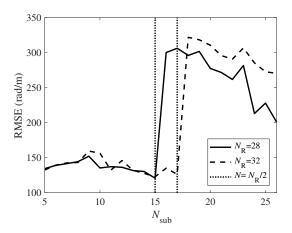
**Figure 3.** Dependence of the proposed method on sub-array size. The black solid line and the dotted line show the results for arrays composed of different numbers of receivers. The vertical black dotted lines show the horizontal values with  $N = N_R/2$ , i.e.,  $N_{sub} - 1 = N_R/2$ .
