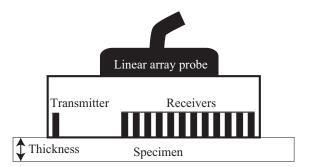
**Figure 1.** System model used in this study. In this study, we used a 4-mm-thick copper (homogeneous isotropic) plate and a 4-mm-thick bone mimicking (transversely isotropic) plate.
