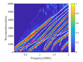
**Figure 5.** Wavenumbers of the 4-mm-thick copper plate estimated using the proposed method and the conventional SVD method. Red dots show the estimates obtained using the proposed method. The color intensity map shows the results obtained using the conventional SVD method. Solid white lines show the theoretical curves.
