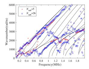
**Figure 11.** Wavenumbers estimated for differently sized sub-arrays. Red cross marks and blue circles show the results obtained for  $N_{sub} = 5$  and 26, respectively. Black lines show the theoretical curves.
