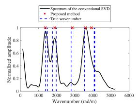
**Figure 8.** Depiction of the wavenumbers obtained using the proposed method and the spectrum obtained using the conventional method at 1.0 MHz. This is the cross-sectional view at the white dotted line shown in Figure 7. The vertical blue dotted lines indicate the theoretical values.
