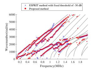
**Figure 10.** Wavenumbers of the 4-mm-thick bone-mimicking plate estimated using the conventional ESPRIT algorithm at a fixed threshold of -30 dB and the proposed method. Red dots show the estimates obtained using the proposed method and blue cross marks show the estimates obtained using the conventional method. Solid gray lines show the theoretical curves.
