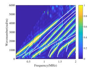
**Figure 4.** Wavenumbers of the 4-mm-thick copper plate estimated using the conventional singular value decomposition (SVD) method. The color intensity map shows the results obtained using the conventional SVD method. Solid white lines show the theoretical curves.
