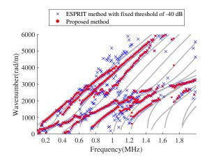
**Figure 9.** Wavenumbers of the 4-mm-thick bone-mimicking plate estimated using the conventional estimation of signal parameters via rotational invariance technique (ESPRIT) algorithm at a fixed threshold of -40 dB and the proposed method. Red dots show the estimates obtained using the proposed method and blue cross marks show the estimates obtained using the conventional method. Solid gray lines show the theoretical curves.
