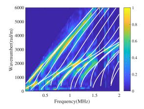
**Figure 6.** Wavenumbers of the 4-mm-thick bone-mimicking plate estimated using the conventional SVD method. The color intensity map shows the results obtained using the conventional SVD method. Solid white lines show the theoretical curves.
