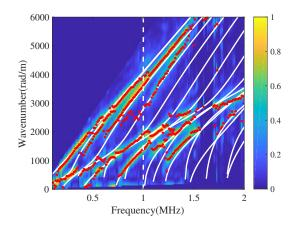
**Figure 7.** Wavenumbers of the 4-mm-thick bone-mimicking plate estimated using the proposed method and the conventional SVD method. Red dots show the estimates obtained using the proposed method. The color intensity map shows the results obtained using the conventional SVD method. Solid white lines show the theoretical curves.
