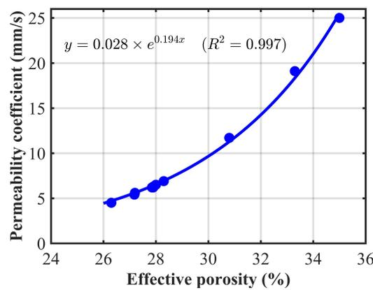
Figure 7. Effective porosity vs. permeability.
