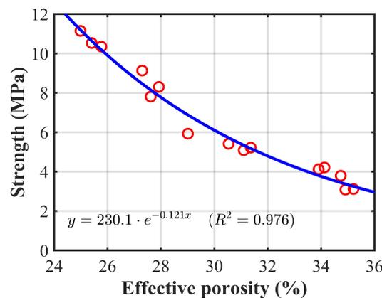
Figure 8. Effective porosity vs. strength.
