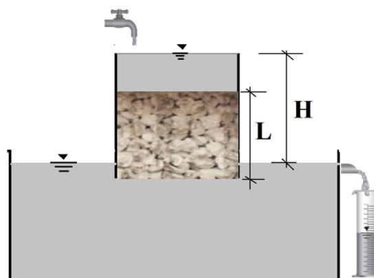
**Figure 1.** Constant-head permeability test.
