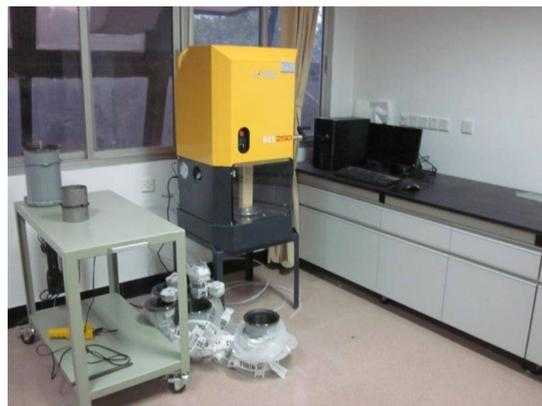
Figure 4. Diagram of the Superpave gyratory compactor used in this paper.
