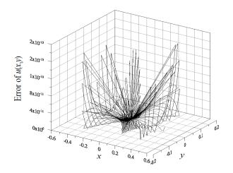
**Figure 3.** The numerical errors of the proposed solution method for the steady-state AC equation with peanut-shaped domain.
