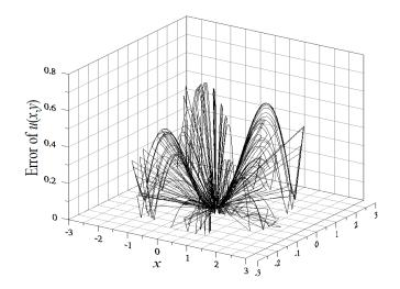
**Figure 17.** The numerical errors of the proposed method solution for the steady-state AC equation with the gear shaped irregular domain.
