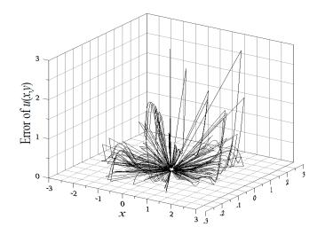
**Figure 7.** The numerical errors of the proposed method solution for the steady-state AC equation with gear irregular domain.
