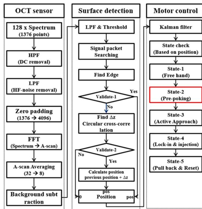
**Figure 3.** Flowchart of OCT data processing for distal sensing and motion control. The processing consists of three main parts: (1) OCT data transformation from measured spectral data, (2) distal information extraction from the OCT data, and (3) motion control based on the distal information. HPF: high-pass filter, LPF: low-pass filter, and FFT: Fast Fourier Transformation.
