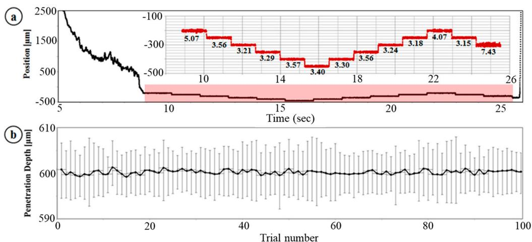
**Figure 6.** (a) Dynamic insertion test under the condition that it has interaction between needle tip and sample material. The upper inserted graph is a partial magnified graph of area in red square in lower entire graph. (b) The average deviation error of 100 injections with error bar consisting a positive and negative RMSE.
