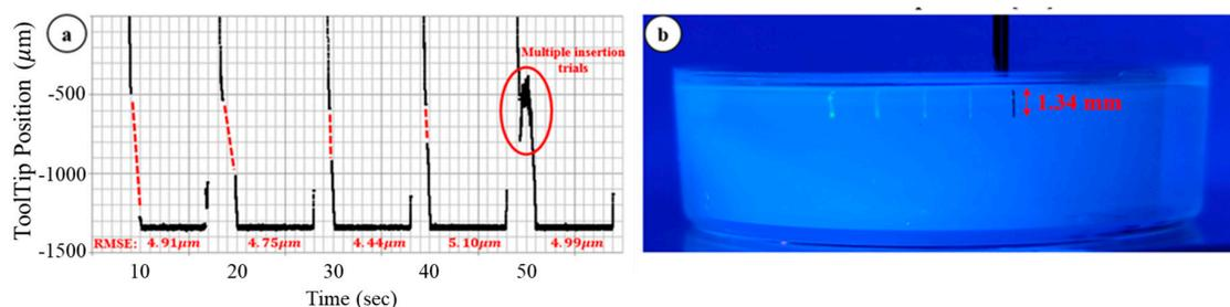
**Figure 4.** Preliminary 10% gelatin phantom injection test: (a) distance tracking data that has blind area caused by surface deformation, (b) five consecutive injection trials on a gelatin sample. The preset penetration depth was 1.34 mm.
