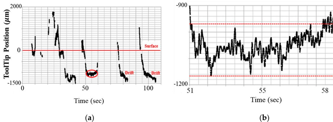
**Figure 1.** Free hand insertion test performed by a retinal surgeon: (a) Needle tip position tracking data during the insertion trial, (b) a magnified area in red ellipse of graph (a). The two red dotted lines mark the range of insertion depth variation during the microinjection.
