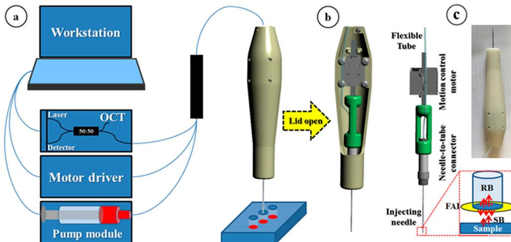
**Figure 2.** (a) System overview of the common-path swept source optical coherence tomography (CP-SSOCT) depth-guided microinjector; (b) internal structure of the microinjector and CP-SSOCT fiberoptic sensor: RB (reflected beam), FAI (Fiber-Air Interface), SB (sample reflected beam); and (c) picture of implemented injector handpiece.
