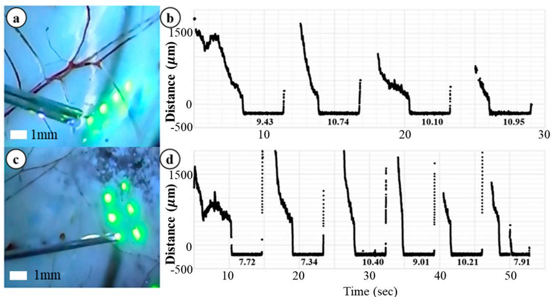
**Figure 7.** The ex-vivo bovine eye injection experiment: (a,c) are snap shots displaying the multiple fluorescein injections. Fluorescein was excited by blue light for fluorescence emission, (b,d) are tracking data of the needle-tip. Each graph has root mean square error (RMSE) below it during depth locking.
