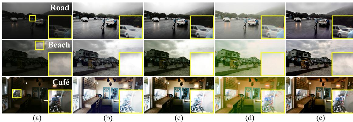
**Figure 15.** Resulting enhanced images of the existing and proposed methods using real low-light images: (a) input image, (b) HE [26], (c) Huang's method [27], (d) Jiang's method [25], and (e) the proposed method.
