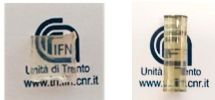
**Figure 2.** Photo of the as-prepared  $90\text{SiO}_2\text{-}10\text{SnO}_2\text{:}0.5\text{Er}^{3+}$  monolithic square with size of  $1 \times 1\text{ cm}^2$  and thickness of  $\approx 0.3\text{ cm}$  and the cylinder with diameter of  $0.5\text{ cm}$  and length of  $1.5\text{ cm}$  obtained after the heat treatment at  $900\text{ }^\circ\text{C}$  for 40 h.
