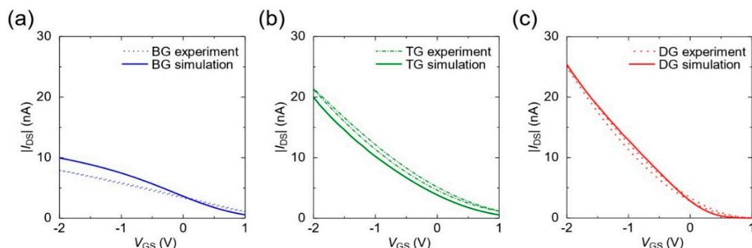
**Figure 3.** Transfer characteristics of (a) bottom-gate, (b) top-gate, and (c) dual-gate OTFTs obtained from the experimental and numerical simulation at  $V_{DS} = -0.1 \text{ V}$ . The channel dimensions were  $W/L = 740 \text{ }\mu\text{m}/7 \text{ }\mu\text{m}$ .
