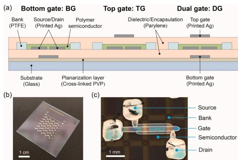
**Figure 1.** (a) Schematic structures, (b) photograph and (c) layout of fabricated organic thin-film transistor (OTFT) devices.
