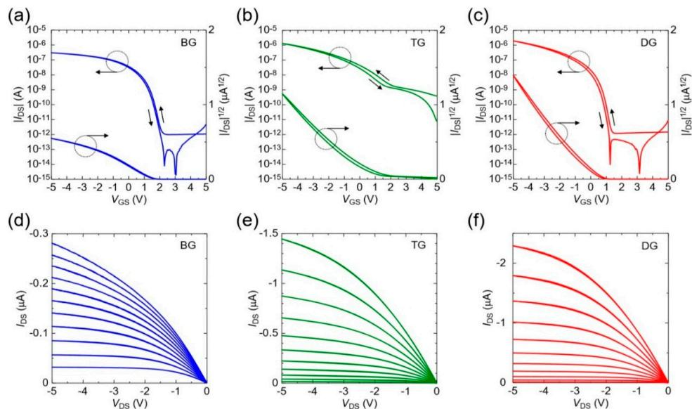
**Figure 2.** Transfer characteristics of fabricated (a) bottom-gate (BG), (b) top-gate (TG), and (c) dual-gate (DG) OTFTs at  $V_{DS} = -5 \text{ V}$ . Output characteristics of fabricated (d) bottom-gate, (e) top-gate, and (f) dual-gate OTFTs. Gate-source voltages were from 0 to  $-5 \text{ V}$  in  $-0.5 \text{ V}$  step. The channel dimensions were  $W/L = 740 \text{ }\mu\text{m}/7 \text{ }\mu\text{m}$ .
