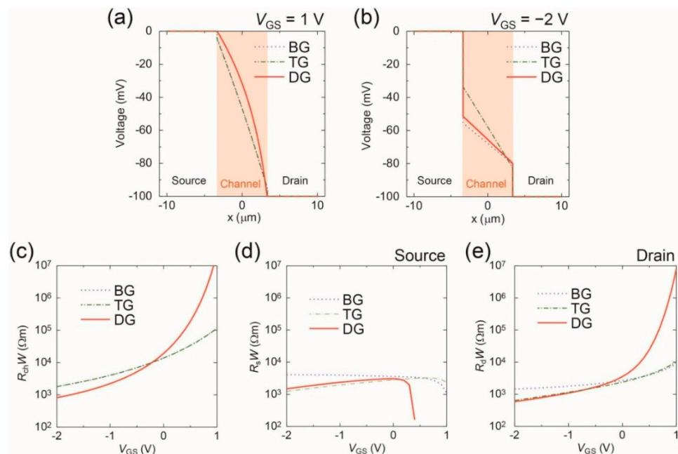
**Figure 5.** Simulation of the potential in source, channel, drain region as a function of  $x$ -axis at (a)  $V_{\text{GS}} = 1 \text{ V}$  and (b)  $V_{\text{GS}} = -2 \text{ V}$ . Channel-width-normalized (c) channel resistance ( $R_{\text{ch}}W$ ), (d) source/channel contact resistance ( $R_sW$ ) and (e) channel/drain contact resistance ( $R_dW$ ) as a function of  $V_{\text{GS}}$ .
