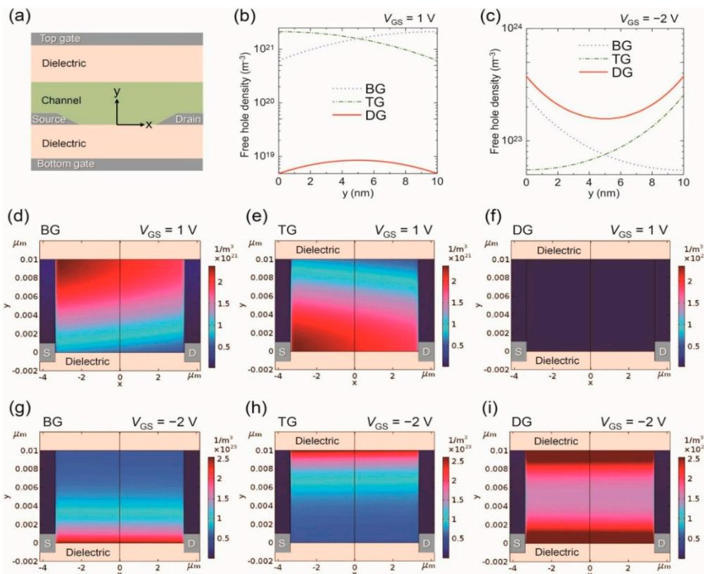
**Figure 4.** (a) Device geometry in the simulation; free hole density as a function of  $y$ -axis at (b)  $V_{GS} = 1$  V and (c)  $V_{GS} = -2$  V. Charge carrier distribution in (d) BG, (e) TG, (f) DG device at  $V_{GS} = 1$  V (off-state), and (g) BG, (h) TG, (i) DG devices at  $V_{GS} = -2$  V (on-state).  $V_{DS} = -0.1$  V.
