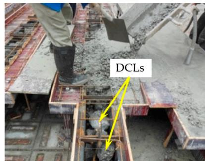
**Figure 4.** Concrete casting of a specimen containing DCLs and FC.
