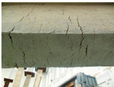
**Figure 10.** Typical surface of fire insulation after the fire test.
