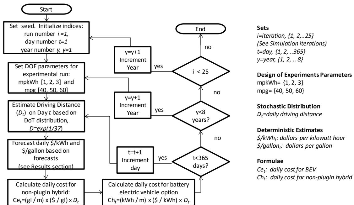
Figure 1. Simulation Flowchart.
