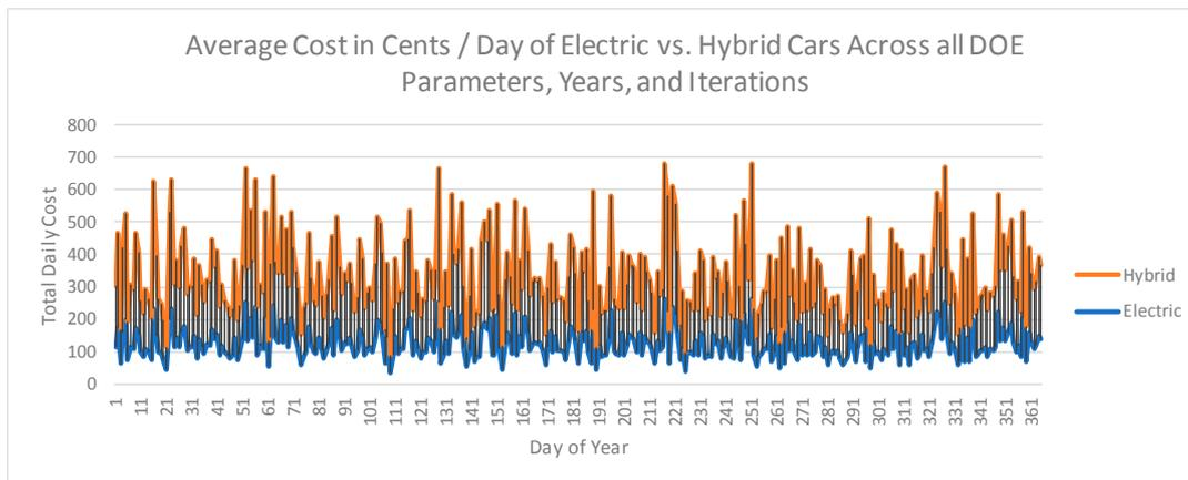
**Figure 6.** Time series for electric vs. hybrid car costs averaged over all design of experiments (DOE) parameters reveal that battery electric vehicles (BEV) variable costs are generally lower than plug-in hybrid electric vehicles (PHEV) costs. The black vertical lines represent the distance between the two cost structures.
