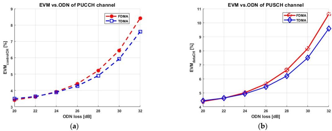
**Figure 14.** Mean EVM vs. ODN loss for 18 NR (200 MHz) channels at 12 dB clipping. (a) PUCCH; (b) PUSCH.
