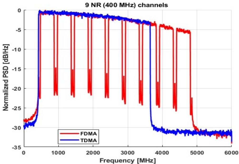
**Figure 9.** Power spectral density of aggregated 9 NR (400 MHz) SCs type 3 channels at the receiver DSP input obtained at 20 dB ODN loss.
