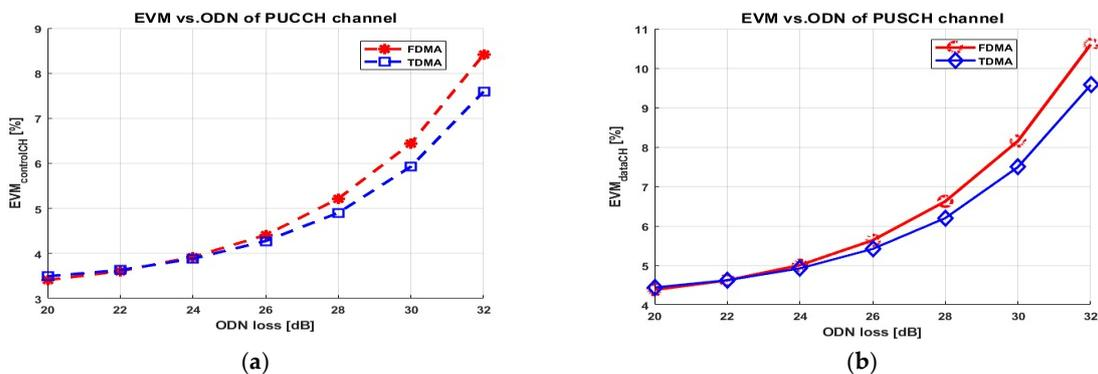
Figure 13. Mean EVM vs. ODN loss for 36 NR (100 MHz) channels at 12 dB clipping. (a) PUCCH; (b) PUSCH.
