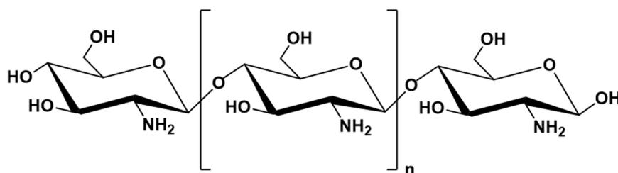
Figure 1. Chitosan chemical structure.
