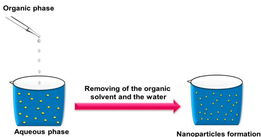
Figure 4. Emulsification solvent diffusion method.
