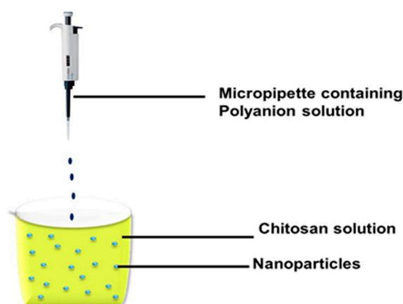
Figure 3. Ionotropic gelation technique.
