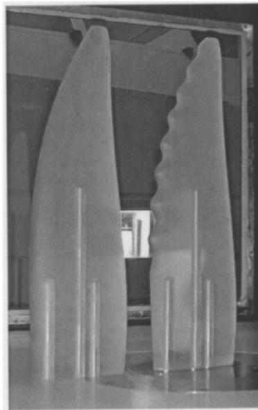
**Figure 7.** 3D scale model of an idealized humpback whale flipper with and without sinusoidal leading edges, reprinted from [60] with permission from AIP Publishing.
