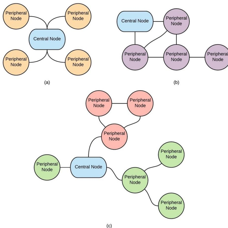
**Figure 2.** Body area network topologies: (a) star topology; (b) mesh topology; and (c) hybrid topology.
