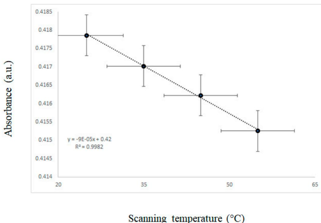
**Figure 3.** Linear regression between absorbance at 280 nm and scanning temperature. Please note that each dot represents the average of all whisky samples scanned at that temperature.
