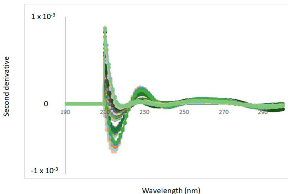
**Figure 2.** Second derivative of UV-VIS spectra of whisky samples scanned at different temperatures (25, 35, 45, and 55 °C).
