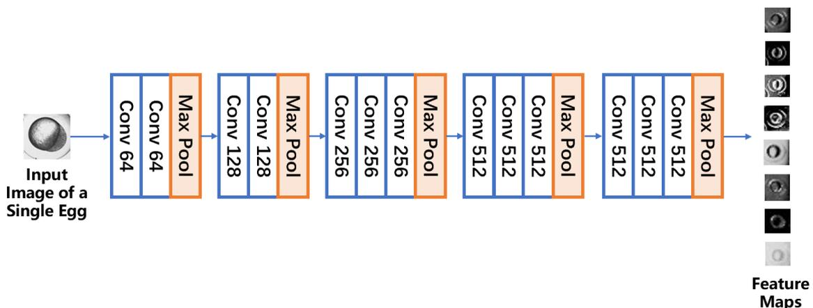
**Figure 5.** The architecture of the convolutional feature extraction network, where ‘Conv N’ stands for a  $3 \times 3$  convolutional layer with N channels, ‘Max Pool’ stands for a  $2 \times 2$  max pooling layer.
