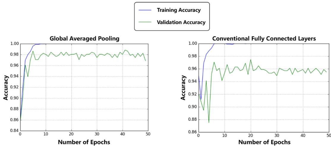
**Figure 6.** The training accuracy curve and validation accuracy curve of both global averaged pooling method and conventional fully connected layers method.
