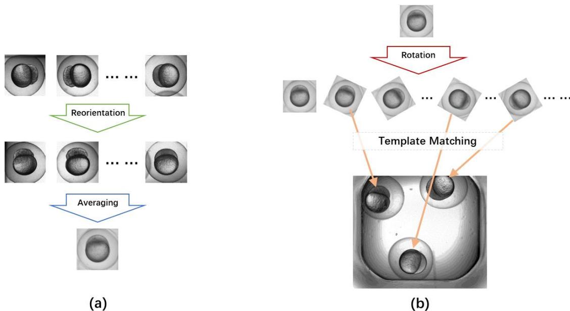
**Figure 3.** The workflow of egg detection. (a) The egg template is created by averaging  $K$  patches of egg samples; (b) The egg template is rotated into different directions, and each rotated patch is moved through the target image to find its matched egg.
