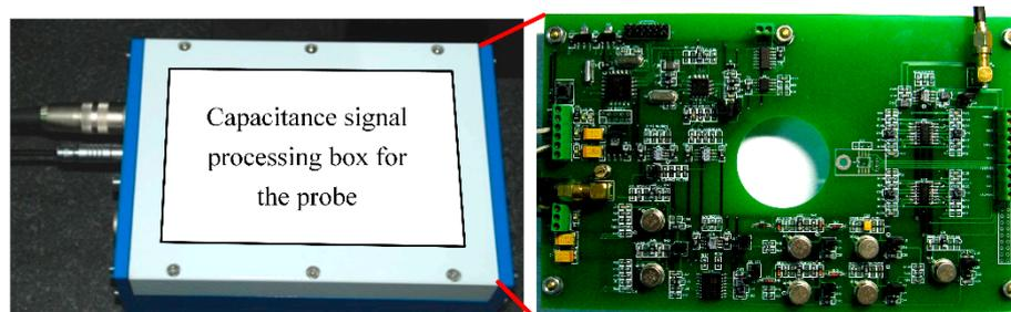
Figure 9. Signal processing circuits and box.
