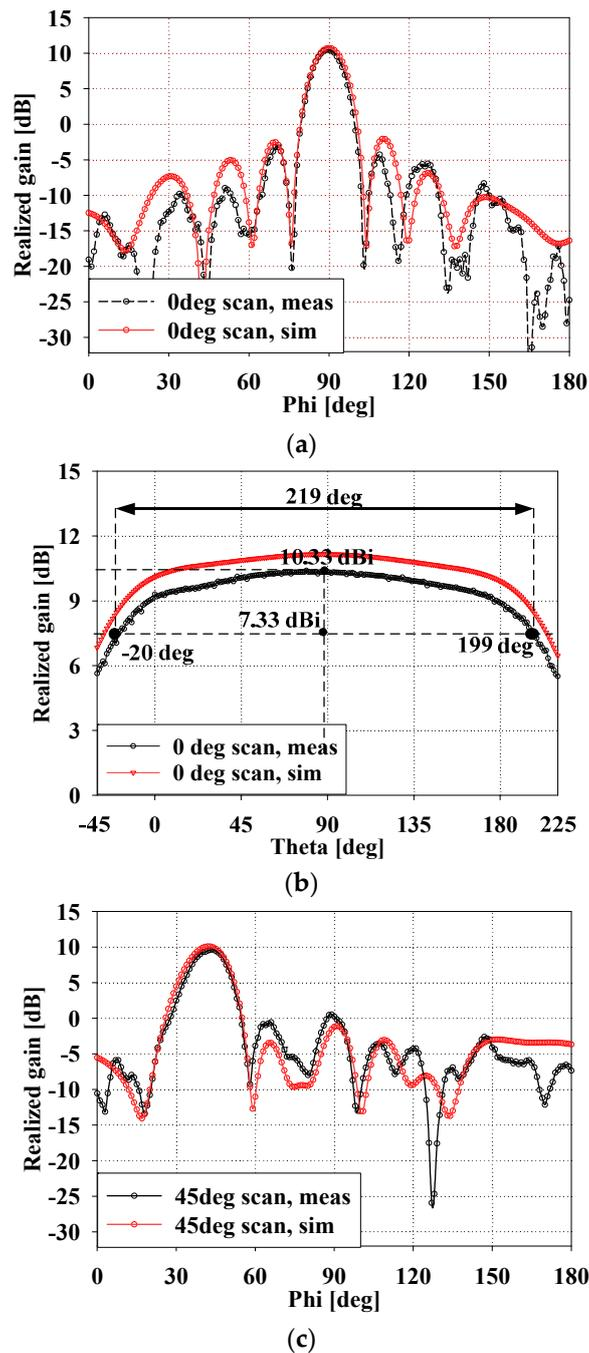
**Figure 14.** Measured and simulated radiation patterns of the proposed array antenna at 28 GHz: (a) XY plane with a 0 degree phase difference; (b) YZ plane with a 0 degree phase difference; (c) XY plane with a 120 degree phase difference.
