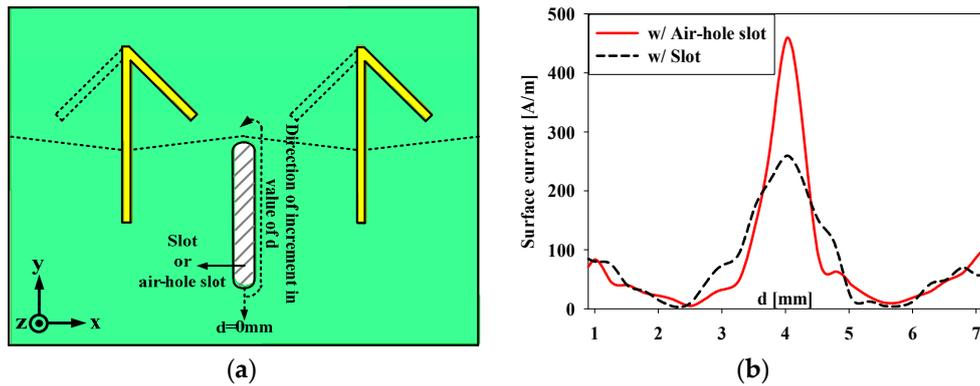
**Figure 6.** Introduction of the air-hole superposed with the slot in the ground: (a) top view of the simulation environment for surface current intensity around the slot (b) comparison of surface current intensity from the supposed two cases.
