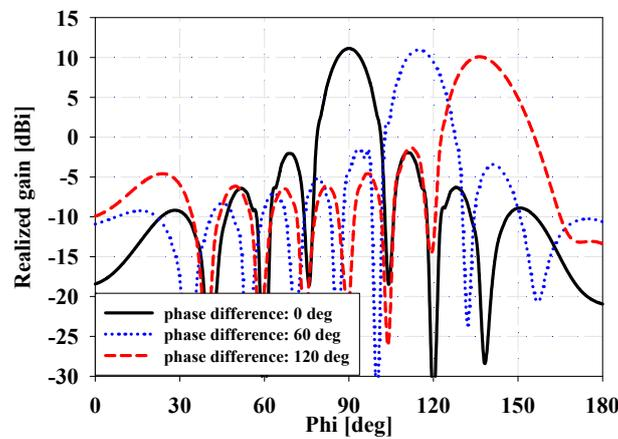
**Figure 11.** Radiation pattern of the proposed phased array antenna at 28 GHz in the XY plane (azimuth) when the phase difference between element ports is varied from 0 degree to 120 degree with a step of 60 degree.
