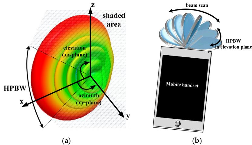
**Figure 1.** The azimuth and elevation plane versus the radiation pattern: (a) half power beam width (HPBW) in the elevation plane and shaded area; (b) hemispheric beam coverage required by mobile handsets.
