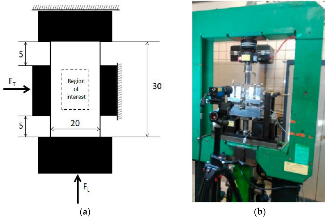
**Figure 2.** (a) Scheme of the loads applied to the specimen, longitudinal forces,  $F_L$ , and transversal forces,  $F_T$ ; (b) picture of the system during experiments. The push-pull testing machine may be observed in the background. The piston and the load cell above, attached to the green frame, can be observed. The system that applies the transversal load can be seen below, while the DIC camera appears in front.
