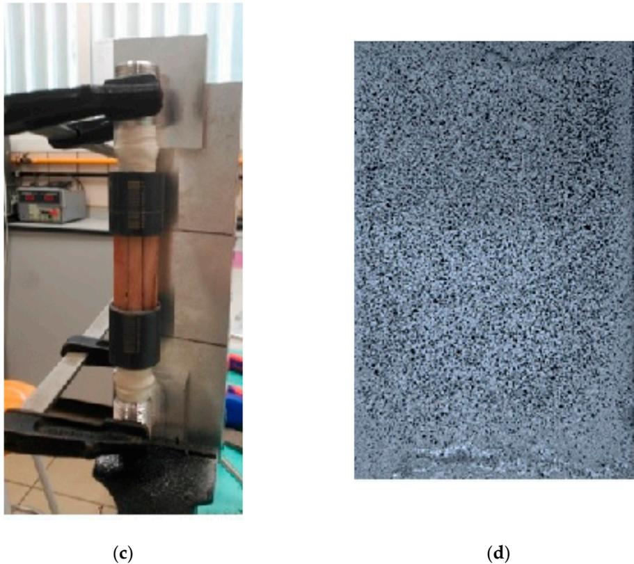
**Figure 1.** (a) Horse femur after extracting a piece from the mid diaphysis for machining; (b) one of the four specimens after milling; (c) embedding process; (d) spray speckle for digital image correlation strain measurements.
