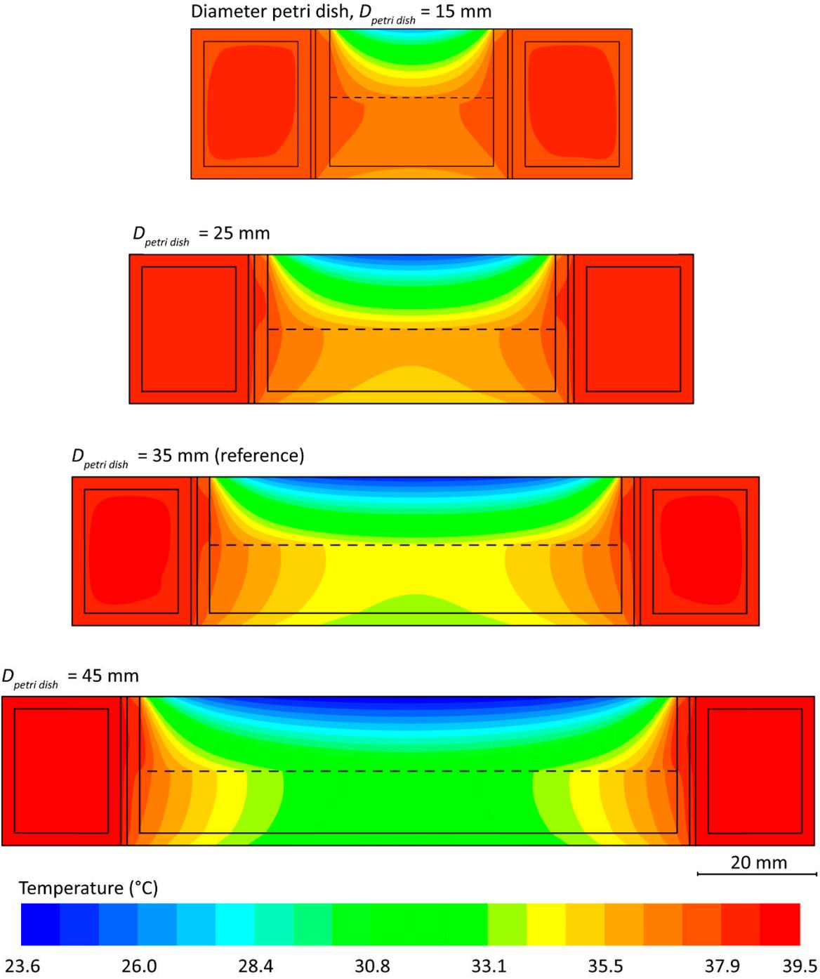
**Figure S6.** Characterizing the thermal performance of the water jacket system with respect to Petri dish diameter ( $D_{Petri\ dish}$ ). The above contours show the temperature distribution along the middle cross section of the Petri dish for  $D_{Petri\ dish}$  values of 15, 25, 35, and 45 mm, as discussed in **Figure 4a**.
