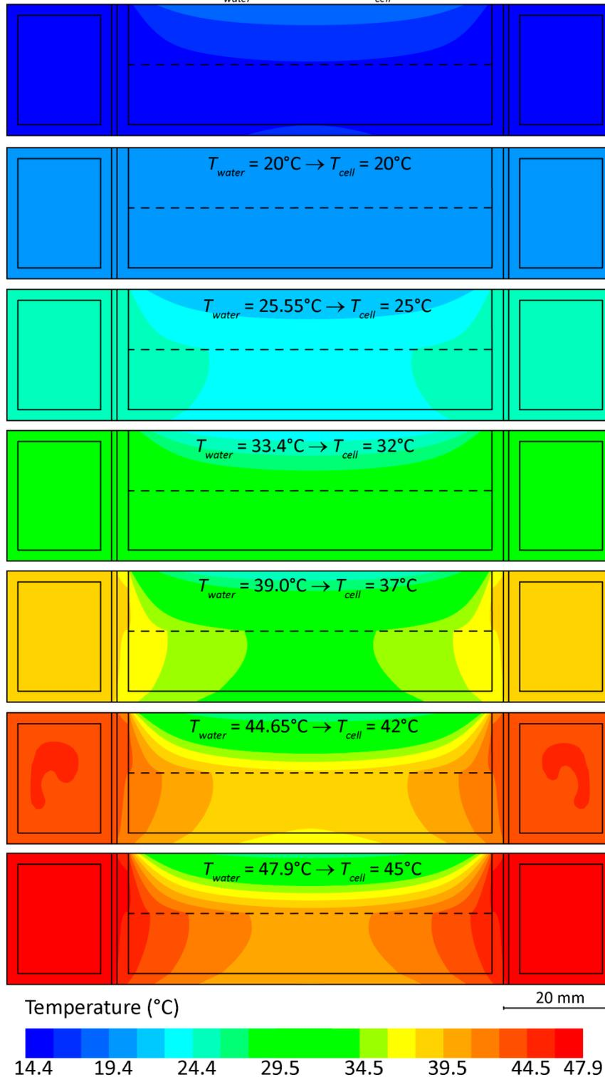
**Figure S3.** Characterizing the thermal performance of the water jacket system with respect to the temperature of the water entering the water jacket ( $T_{water}$ ). The above contours show the temperature distribution along the middle cross section of the Petri dish for  $T_{water}$  values of 14.35, 20, 25.55, 33.4, 39, 44.65 and 47.9 $^{\circ}\text{C}$ , as discussed in **Figure 3b**.
