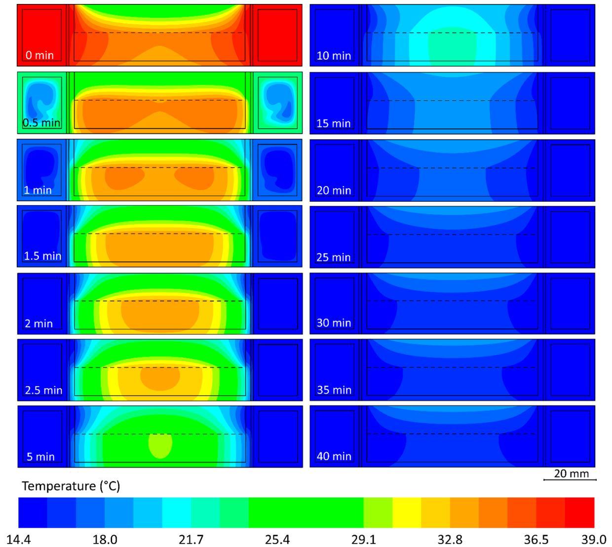
**Figure S18.** Characterizing the dynamic response of the water jacket system when decreasing the water inlet temperature from 39 to 14.35°C at 0 min (corresponding to varying the target sample temperature from 37 to 15°C), as discussed in **Figure 7e**.
