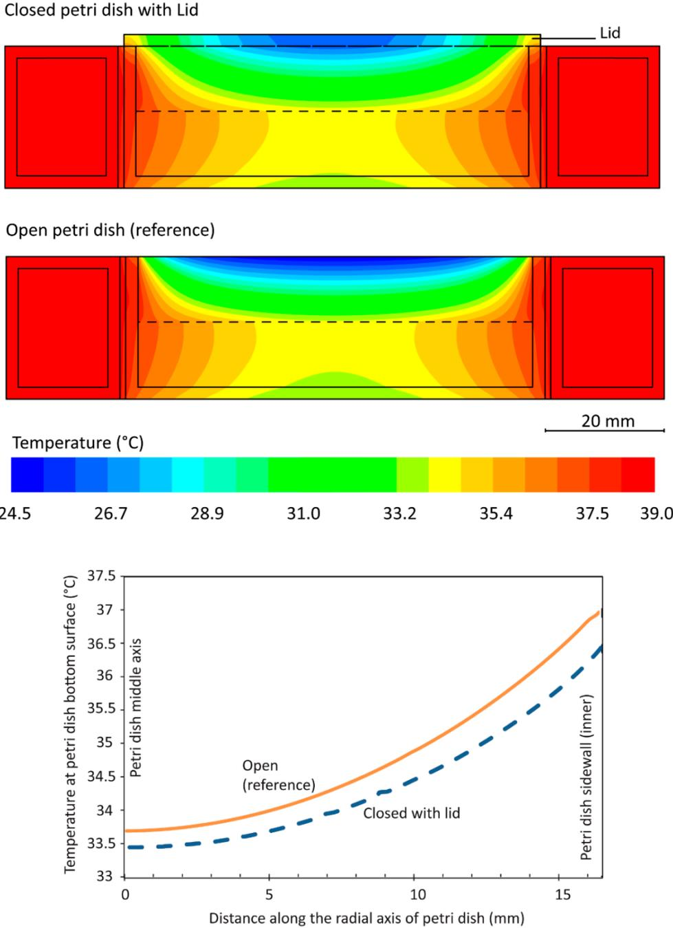
**Figure S14.** Characterizing the thermal performance of the water jacket system in the presence of a polystyrene lid inserted on the top surface of the Petri dish. The above contours show the temperature distribution along the middle cross section of the Petri dish in the presence and absence of the polystyrene lid. The plot compares the temperature profile along the radial axis of the Petri dish in the presence and absence of the lid.
