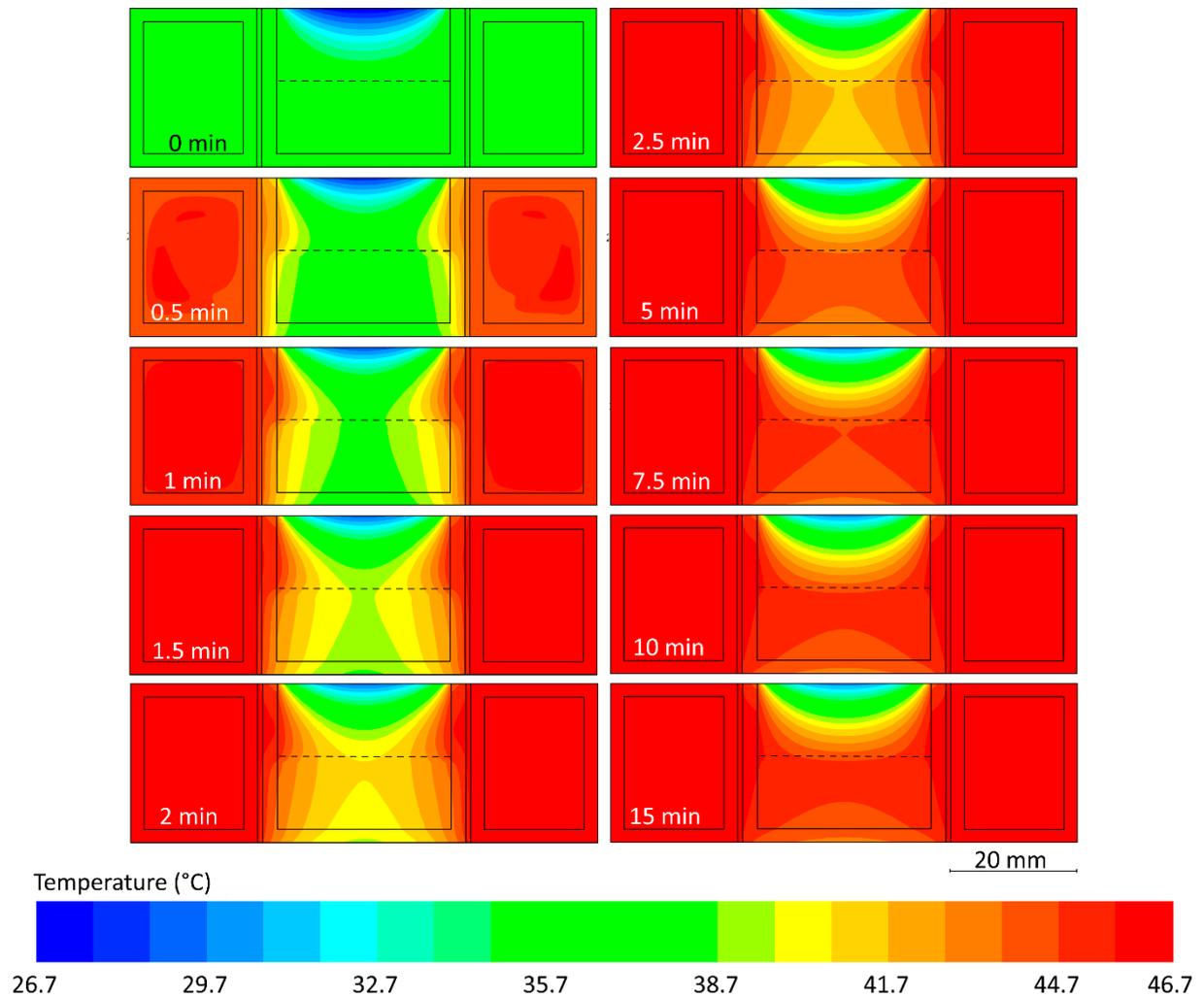
**Figure S20.** Characterizing the dynamic response of the water jacket system with a **Petri dish diameter of 15 mm** when increasing the water inlet temperature from 39 to 46.7°C at 0 min (corresponding to varying the target sample temperature from 37 to 45°C), as discussed in **Figure 8c**.
