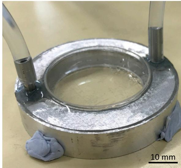
**Figure S1.** Prototype water jacket used for measuring the temperature profile across the top free surface of the Petri dish using an infrared camera.
