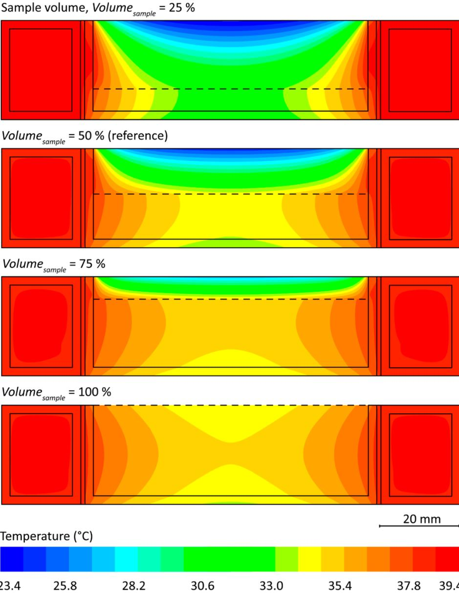
**Figure S7.** Characterizing the thermal performance of the water jacket system with respect to the volume of biological sample added into the Petri dish ( $V_{sample}$ ). The above contours show the temperature distribution along the middle cross section of the Petri dish for  $V_{sample}$  values of 25, 50, 75, and 100%, as discussed in **Figure 4b**. The filled level of the sample inside the Petri dish is shown by dashed line.
