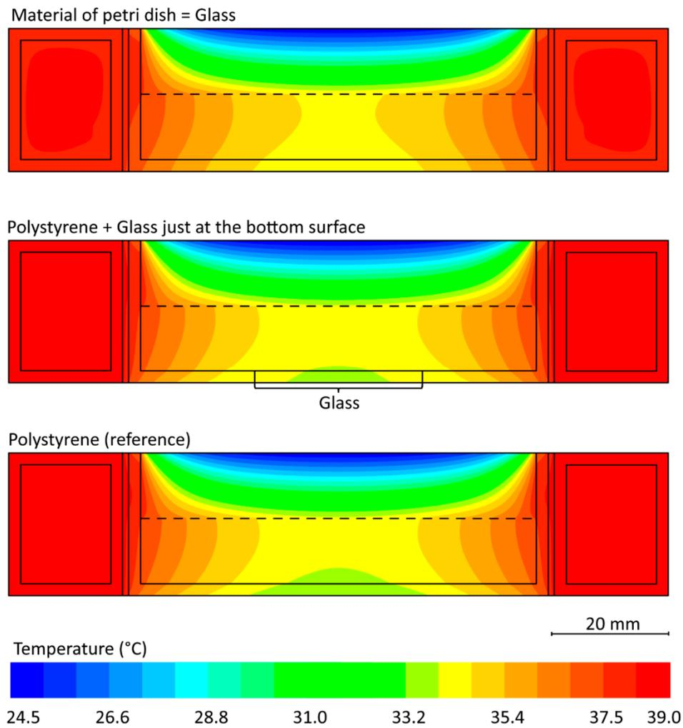
**Figure S8.** Characterizing the thermal performance of the water jacket system with respect to the material of Petri dish. The above contours show the temperature distribution along the middle cross section of the Petri dish for the cases of fully polystyrene, polystyrene-glass, and fully glass, as discussed in **Figure 4c**.
