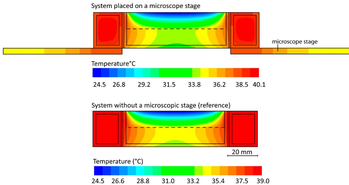
**Figure S12.** Characterizing the thermal performance of the water jacket system in the presence of a microscopic stage made of stainless steel with a thermal conductivity of 16.5 W/mK. The above contours show the temperature distribution along the middle cross section of the Petri dish in the absence and presence of a microscopic stage made of stainless steel with internal and external diameters of 36 and 115 mm and a thickness of 2 mm.
