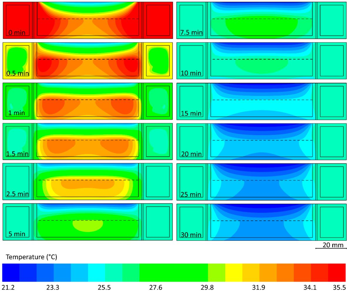
**Figure S25.** Characterizing the dynamic response of the water jacket by setting the localised heat transfer coefficient at the bottom surface of the Petri dish bottom to 20 W/m<sup>2</sup>K along with decreasing the water inlet temperature from 39 to 30.7°C at 0 min (corresponding to varying the target sample temperature from 37 to 29°C), as discussed in **Figure 8g**.
