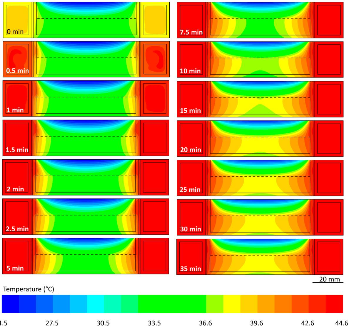
**Figure S16.** Characterizing the dynamic response of the water jacket system when increasing the water inlet temperature from 39.0 to 44.6°C at 0 min (corresponding to varying the target sample temperature from 37 to 42°C), as discussed in Figure 7e.
