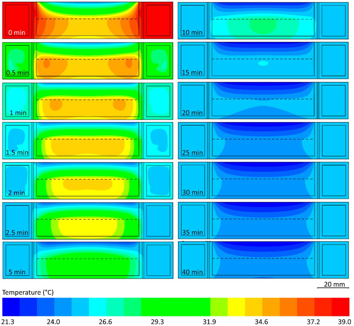
**Figure S17.** Characterizing the dynamic response of the water jacket system when decreasing the water inlet temperature from 39 to 25.55°C at 0 min (corresponding to varying the target sample temperature from 37 to 25°C), as discussed in **Figure 7e**.
