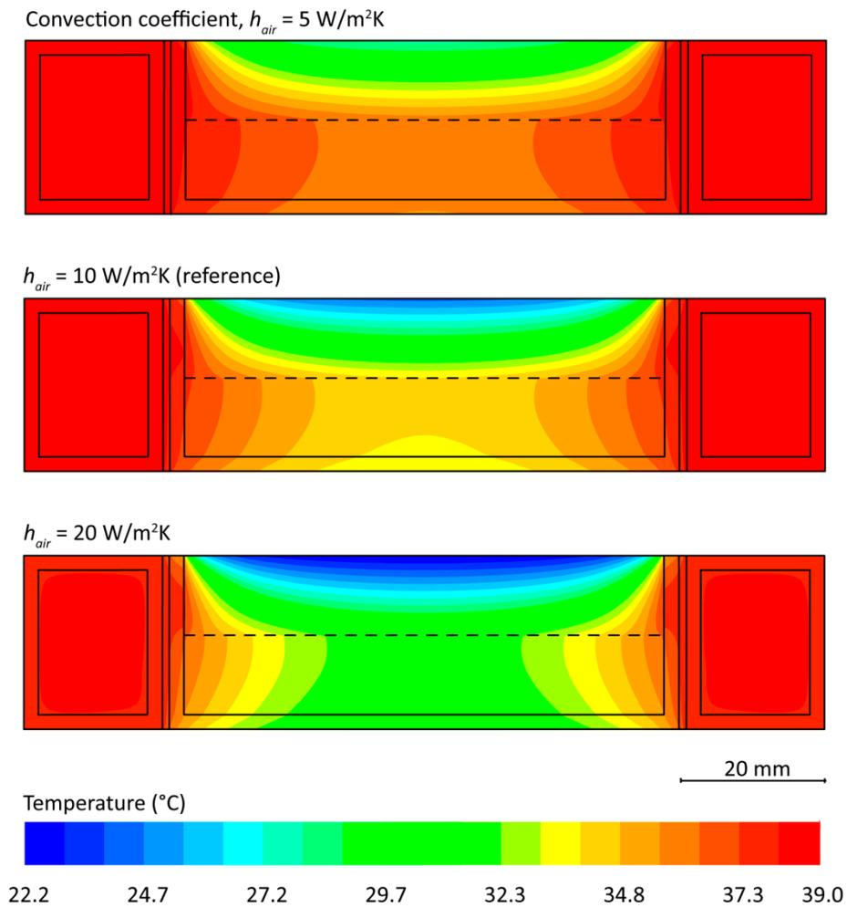
**Figure S5.** Characterizing the thermal performance of the water jacket system with respect to the convective heat transfer coefficient of ambient ( $h_{air}$ ). The above contours show the temperature distribution along the middle cross section of the Petri dish for  $h_{air}$  values of 5, 10, and 20  $\text{W/m}^2\text{K}$ , as discussed in **Figure 3d**.
