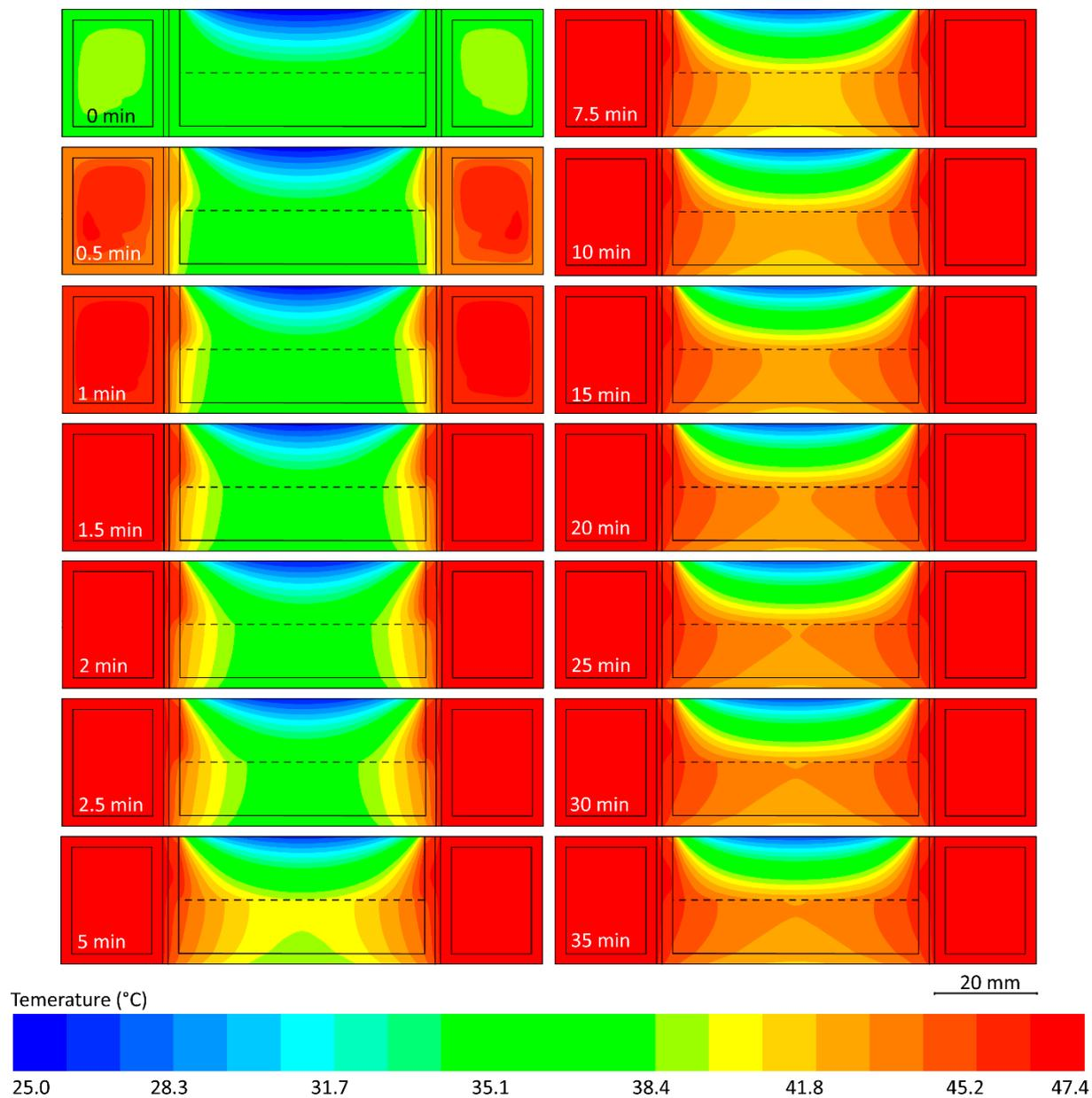
**Figure S21.** Characterizing the dynamic response of the water jacket system with a **Petri dish diameter of 25 mm** when increasing the water inlet temperature from 39 to 47.4°C at 0 min (corresponding to varying the target sample temperature from 37 to 45°C), as discussed in **Figure 8c**.
