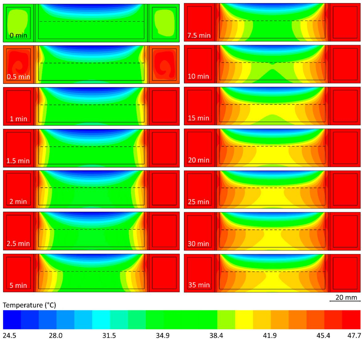
**Figure S19.** Characterizing the dynamic response of the water jacket system when increasing the water inlet temperature from 39 to 47.7°C at 0 min (corresponding to varying the target sample temperature from 37 to 45°C) at a water flow rate of 120 mL/min recirculating through the water jacket), as discussed in **Figure 8b**.
