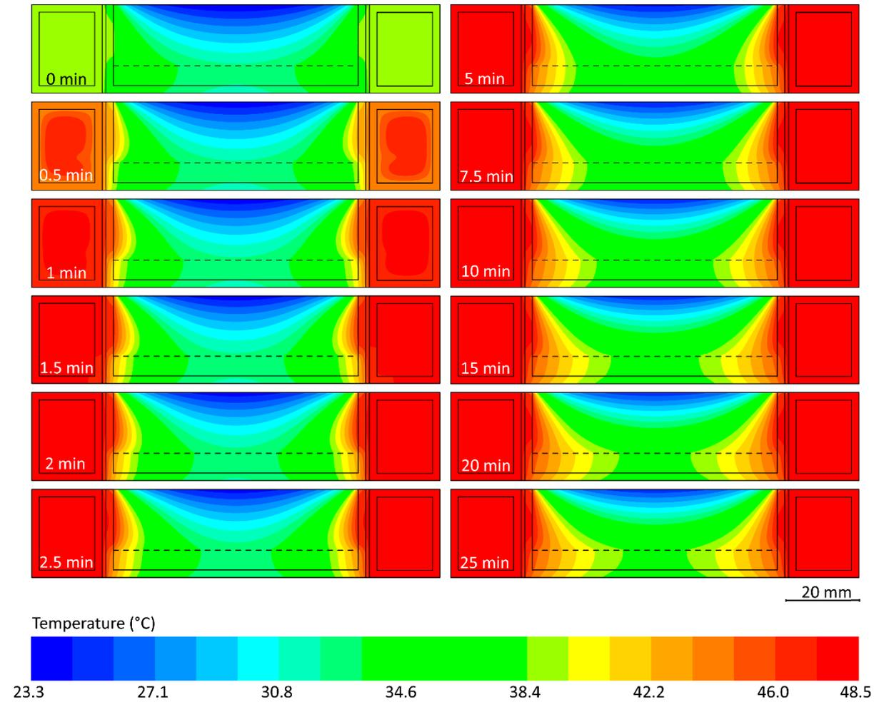
**Figure S22.** Characterizing the dynamic response of the water jacket with a **sample volume of 25%** inside the Petri dish (shown with dashed line) when increasing the water inlet temperature from 39 to 48.5°C at 0 min (corresponding to varying the target sample temperature from 37 to 45 C), as discussed in **Figure 8d**.
