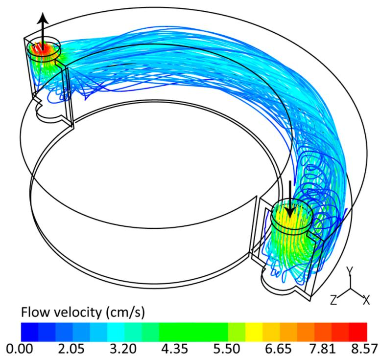
**Figure S11.** Flow streamlines along the semi-circular water jacket chamber coloured by velocity magnitude (cm/s), water is applied into the chamber at 60 mL/min, as discussed in **Figure 5b**.
