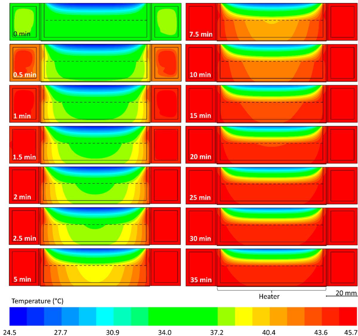
**Figure S24.** Characterizing the dynamic response of the water jacket with a **heater implemented underneath the Petri dish** producing 265 mW along with increasing the water inlet temperature from 39 to 45.7°C at 0 min (corresponding to varying the target sample temperature from 37 to 45°C), as discussed in **Figure 8f**.
