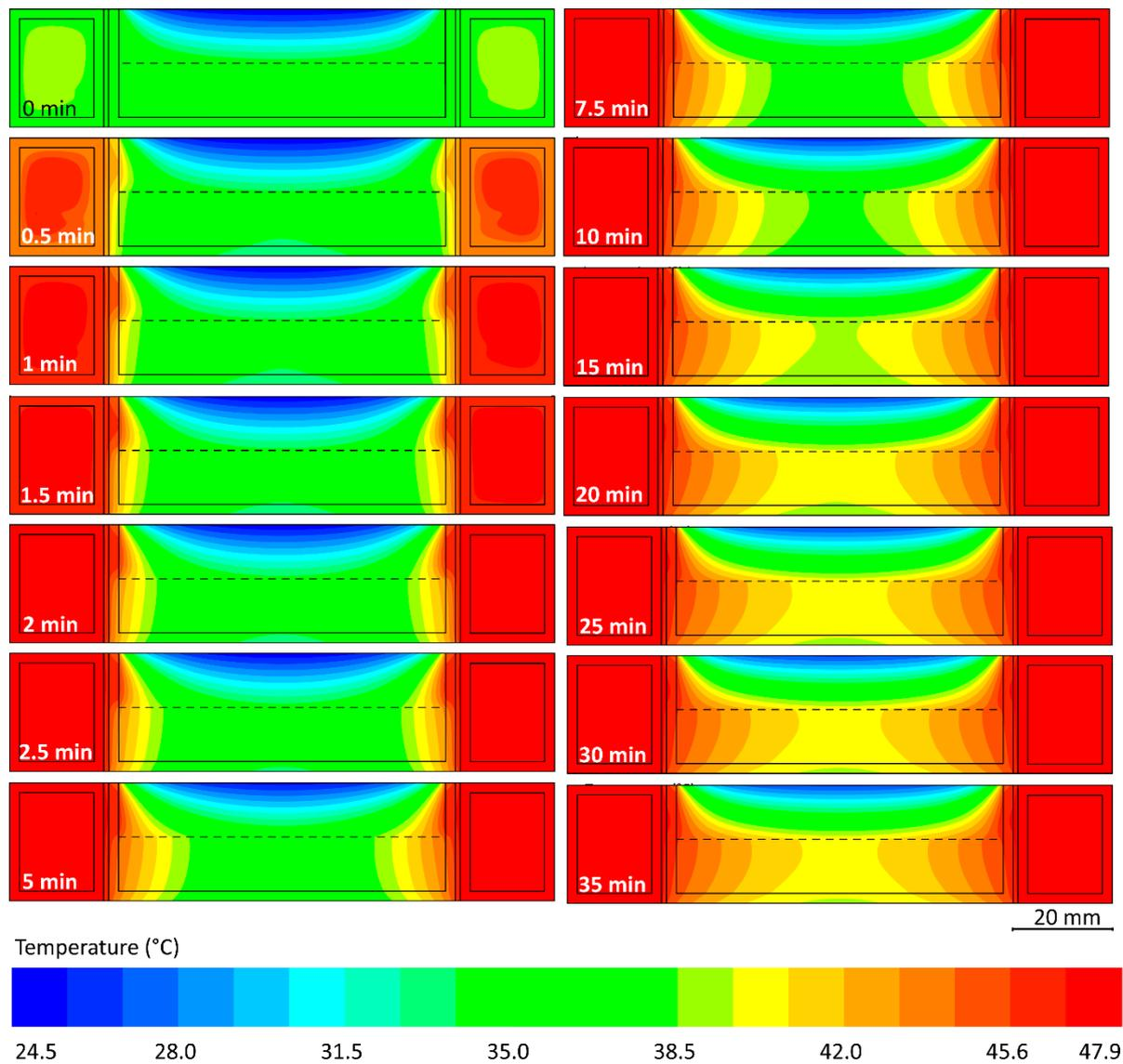
**Figure S15.** Characterizing the dynamic response of the water jacket system when increasing the water inlet temperature from 39.0 to 48.5°C at 0 min (corresponding to varying the target sample temperature from 37 to 45°C), as discussed in Figures 7b-d.
