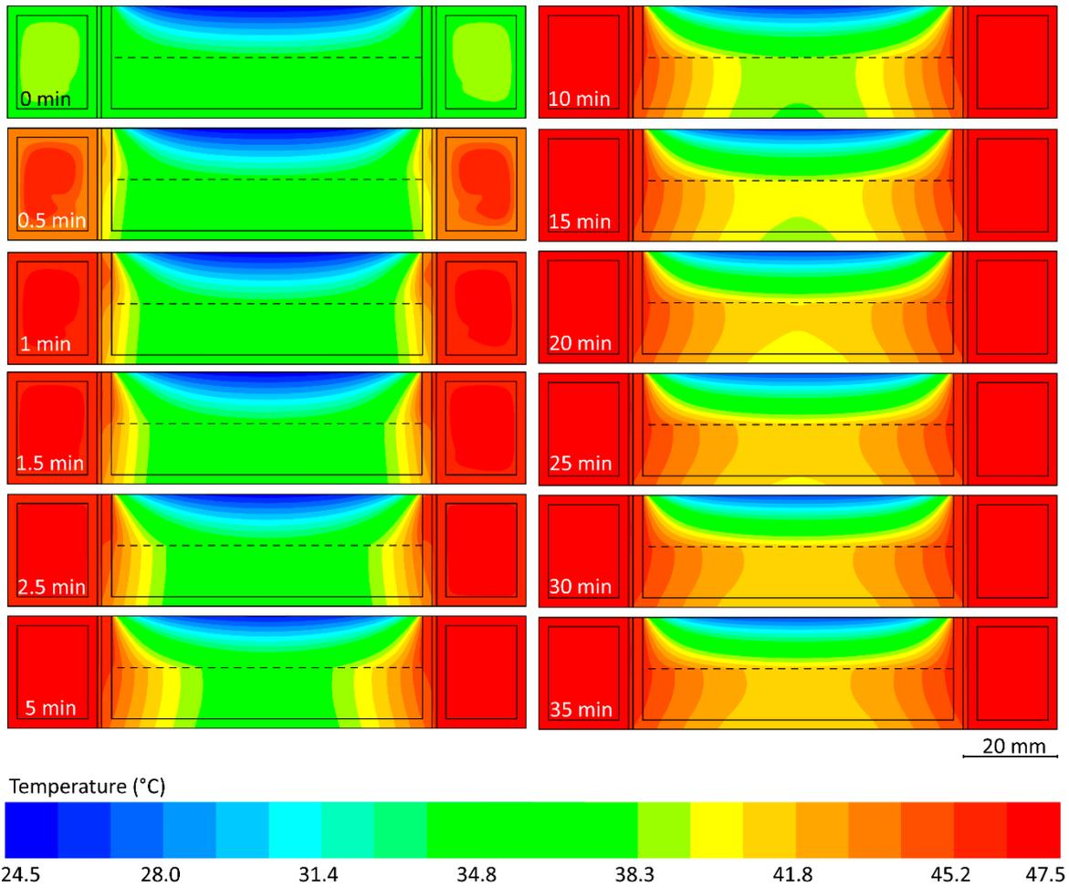
**Figure S23.** Characterizing the dynamic response of the water jacket with a **glass Petri dish** when increasing the water inlet temperature from 39 to 47.5°C at 0 min (corresponding to varying the target sample temperature from 37 to 45°C), as discussed in **Figure 8e**.
