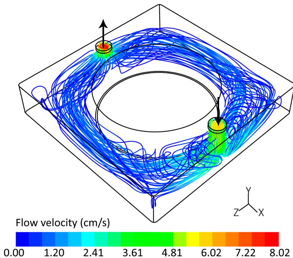
**Figure S10.** Flow streamlines along the square water jacket chamber coloured by velocity magnitude (cm/s), water is applied into the chamber at 60 mL/min, as discussed in **Figure 5a**.
