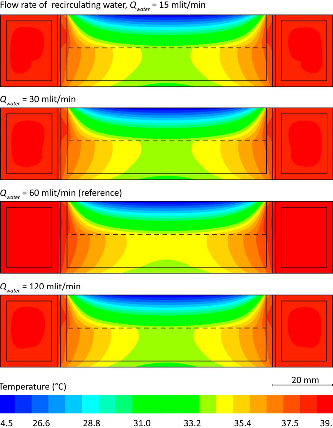
**Figure S2.** Characterizing the thermal performance of the water jacket system with respect to the flow rate of the water recirculating through the water jacket ( $Q_{water}$ ). The above contours show the temperature distribution along the middle cross section of the Petri dish for  $Q_{water}$  values of 15, 30, 60 and 120 mL/min, as discussed in **Figure 3a**.
