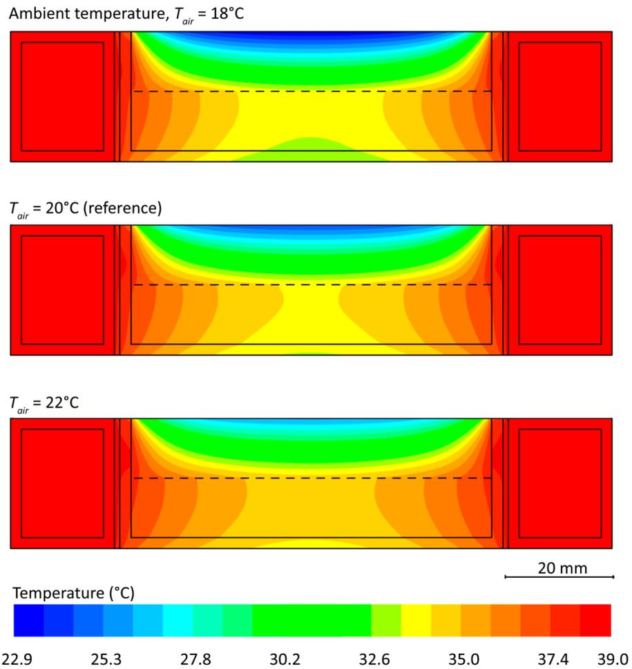
**Figure S4.** Characterizing the thermal performance of the water jacket system with respect to the temperature of the ambient air ( $T_{air}$ ). The above contours show the temperature distribution along the middle cross section of the Petri dish for  $T_{air}$  values of 18, 20 and  $22^\circ\text{C}$ , as discussed in **Figure 3c**.
