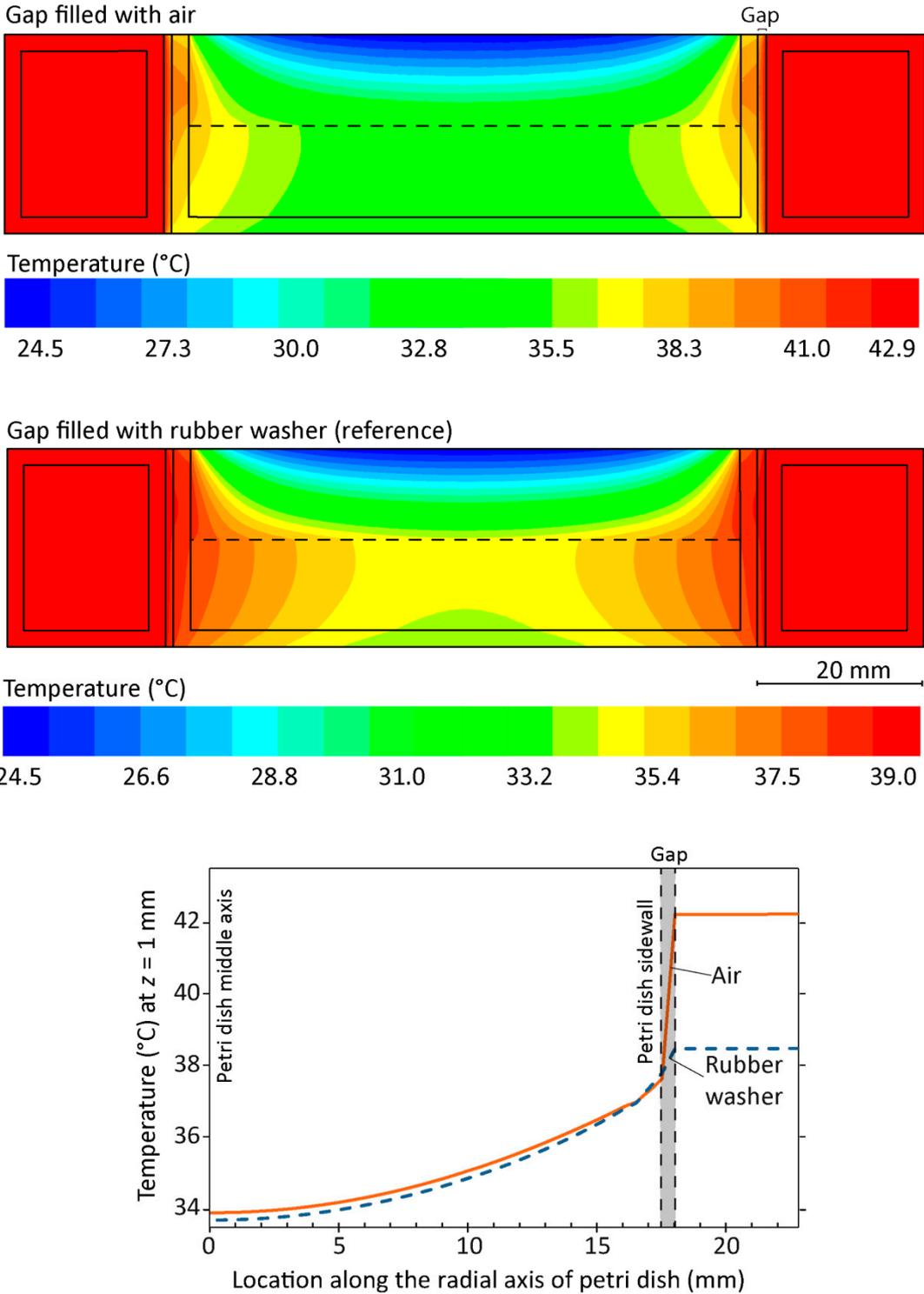
**Figure S13.** Characterizing the thermal performance of the water jacket system with respect to the material inserted between the Petri dish and the water jacket. The above contours show the temperature distribution along the middle cross section of the Petri dish for the cases of air and rubber washer. The plot compares the temperature profile along the radial axis of the Petri dish.
