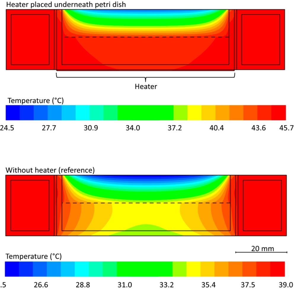
**Figure S9.** Characterizing the thermal performance of the water jacket system in the presence of a heater implemented underneath the Petri dish. The above contours show the temperature distribution along the middle cross section of the Petri dish in the absence and presence of a heater producing 187 mW, as discussed in **Figure 4d**.
