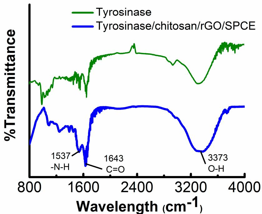
**Figure S1.** The ATR- FTIR spectra of chitosan-modified electrode with tyrosinase (blue line) and spectra of tyrosinase alone (green line).
