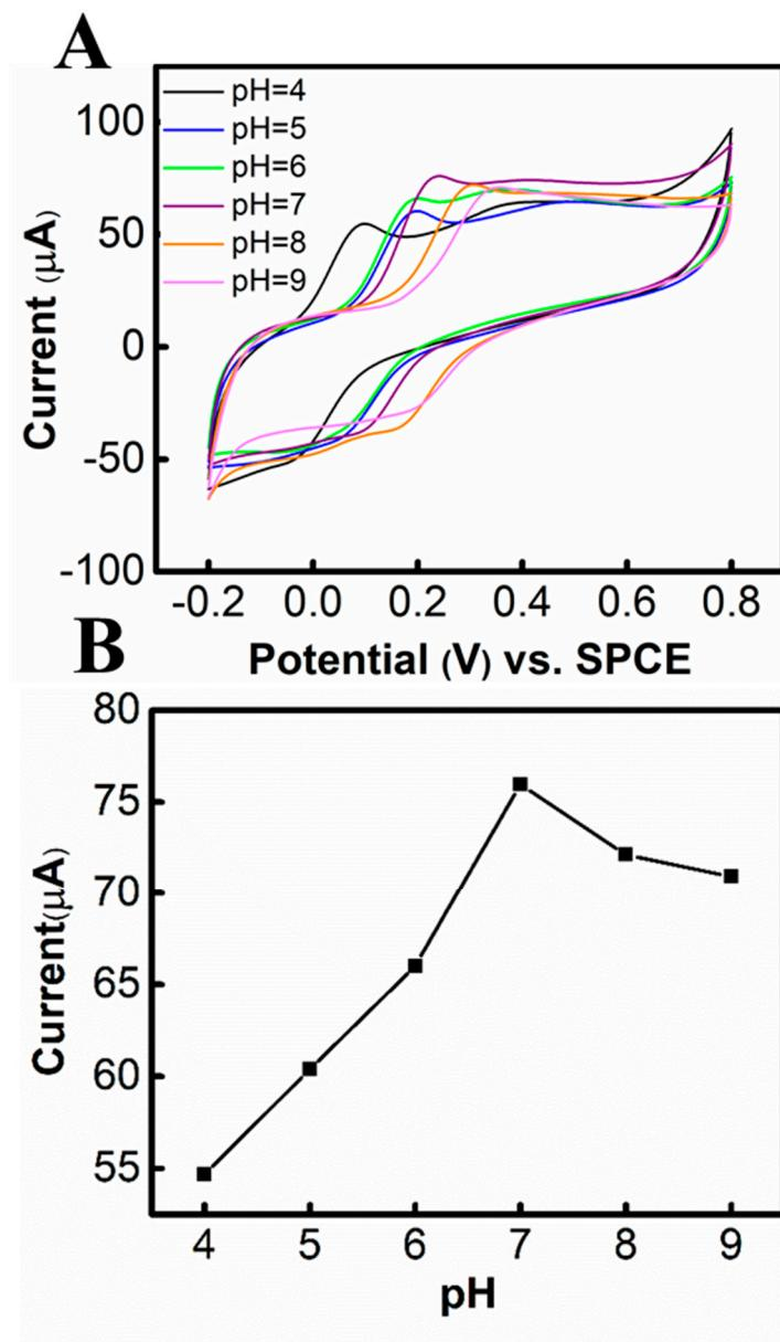
**Figure S4.** (A) CV curves and (B) current response (at a scan rate of  $100 \text{ mVs}^{-1}$ ) vs. various pH levels of tyrosinase/chitosan/rGO/SPCE. Dopamine (DA) concentration was  $1 \text{ mM}$  in  $10 \text{ mM}$  phosphate buffer.
