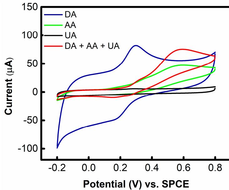
**Figure S5.** CV curves of chitosan/rGO/SPCE in the presence of DA (100  $\mu\text{M}$ ), Ascorbic acid (AA) (100  $\mu\text{M}$ ), Uric acid (UA) (100  $\mu\text{M}$ ), and a mixture of three.
