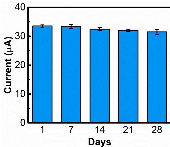
**Figure S6.** Stability of tyrosinase/chitosan/rGO/SPCE. Error bars represent the standard deviation from triplicate measurements.
