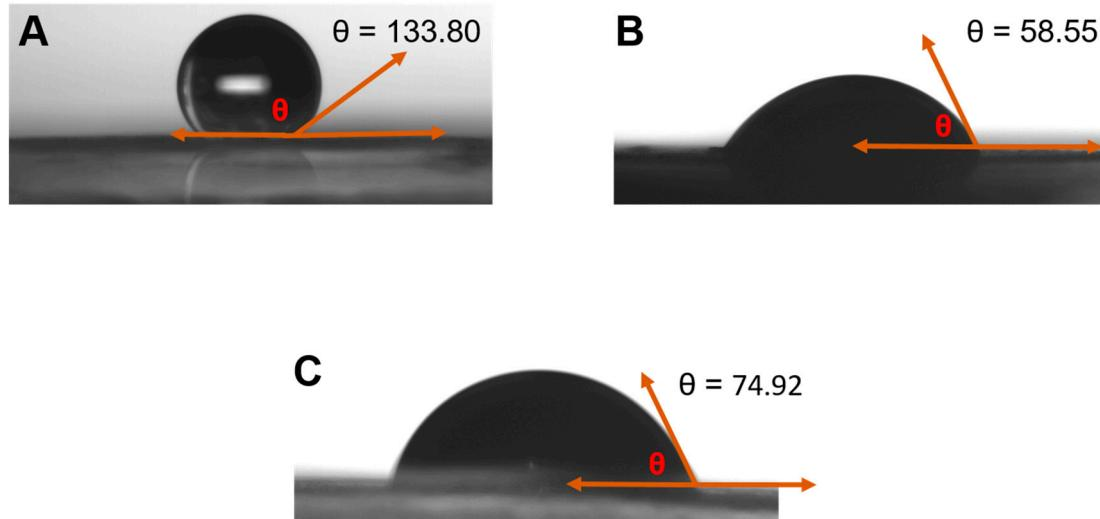
**Figure S2.** Contact angles of different electrode surfaces. (A) reduced graphene oxide (rGO)/screen-printed carbon electrode (SPCE), (B) chitosan/rGO/SPCE, and (C) tyrosinase/chitosan/rGO/SPCE.
