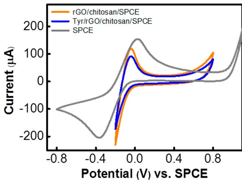
**Figure S3.** Cyclic voltammetry (CVs) (at a scan rate of  $100 \text{ mVs}^{-1}$ ) of different electrodes in a standard redox system containing  $5 \text{ mM Fe}[\text{CN}_6]^{4-}$  in  $0.1 \text{ M KCl}$ .
