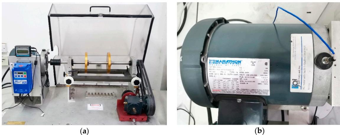
**Figure 17.** (a) Mechanical equipment failure simulation (MFS) test bench; (b) Fault motor.
