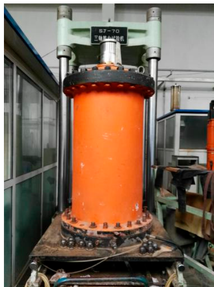
Figure 4. Large-scale triaxial shear test.
