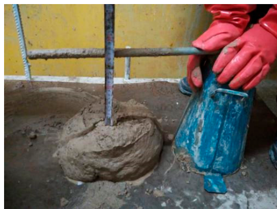
Figure 2. Slump test at the construction site.
