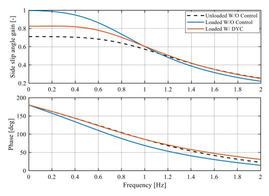
Figure 8. Frequency response of side slip angle with respect to front steering angle.
