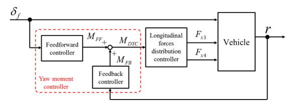
Figure 4. Block diagram of the DYC system.
