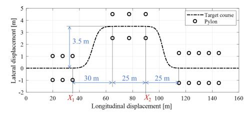
Figure 14. Target course of the double-lane change test.
