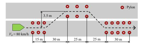
Figure 18. Condition of the double-lane change test course.
