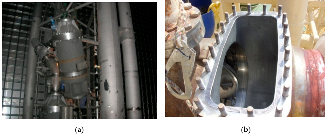
Figure 1. Examples of liquefied natural gas (LNG) cargo containment system maintenance tasks during dry docking. (a) Detaching a cargo pump in an LNG cargo tank for an overhaul inspection. The inside of the LNG cargo tank should be prepared as a nonhazardous working environment after inerting, warming, and aerating. (b) Butterfly LNG cargo valve inspection after inerting, warming, and aerating for safe repair.
