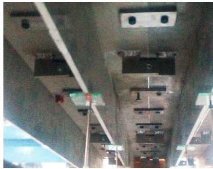
Figure 13. Photo of the devices designed to simulate the damage of the transverse connection between the two T-shaped beams.
