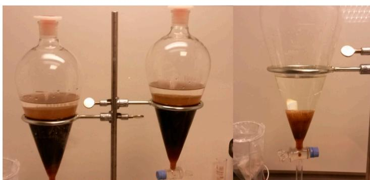
**Figure 1.** Hexane extraction step. Three zones are formed: Top: hexane; intermediate: hexane and unsaturated fat; bottom: purified crude glycerol.
