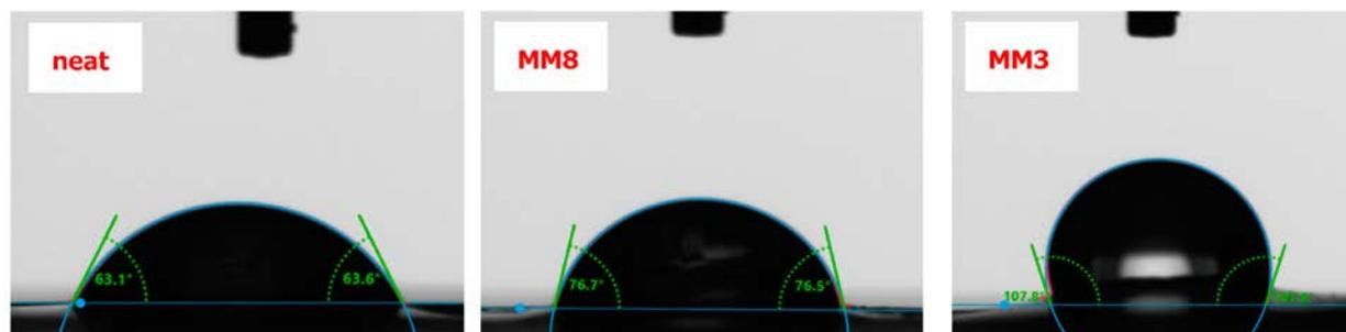
**Figure 6.** Characteristic images of water contact angles on three membrane surfaces.
