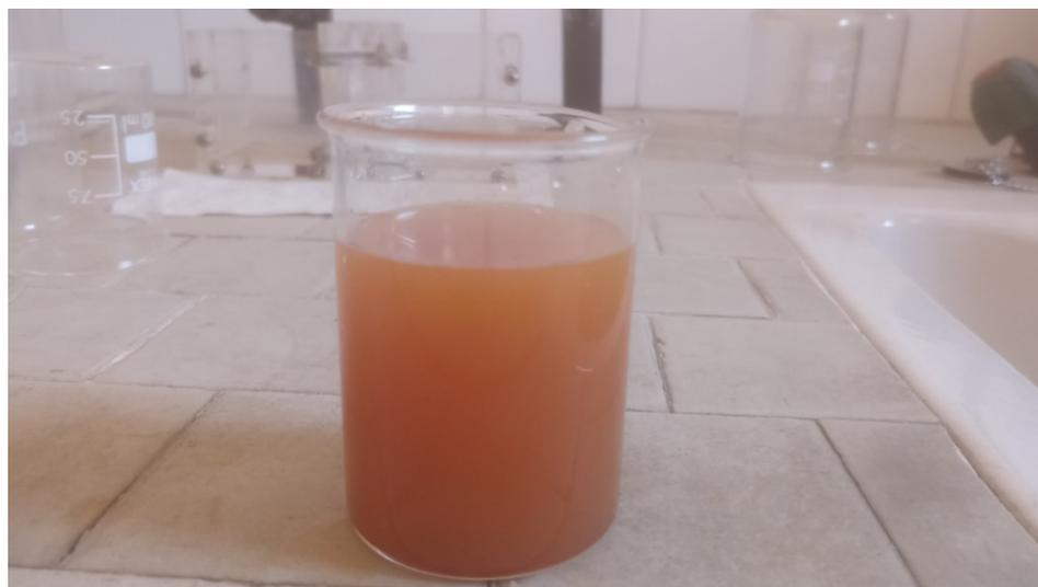
**Figure 1.** Presence of iron(III) in tap water due to degradation of pipelines (picture Alguacil and Robla).
