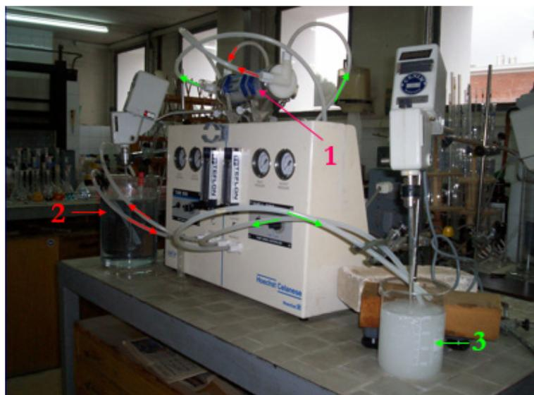
**Figure 2.** View of the hollow fiber module operating in the recycling mode of the phases. (1) Hollow fiber membrane contactor, (2) feed phase tank, and (3) pseudo-emulsion phase tank. Red colour: feed phase flow. Green colour: pseudo-emulsion phase flow.
