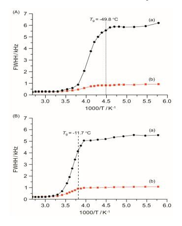
The activation energy,  $E_a$ , of the samples can be obtained from NMR line narrowing data. The NMR motional narrowing of the <sup>7</sup>Li linewidth takes place when the rate of fluctuations of the local magnetic fields or electric field gradients, which are generally described by a correlation time,  $\tau_c$ , is of the order of the rigid lattice linewidth,  $\Delta_{RL}$
