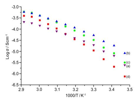
As the conductivity plot suggests a curve profile, necessitating interpretation of the results by the VTF equation:
