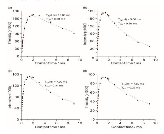
Figure 6. <sup>13</sup>C CPMAS NMR spectra (70.7 ppm) of TIE(600)-Z hybrid electrolytes with Z = (a) 32; (b) 24; (c) 16 and (d) 8, as a function of contact time.
