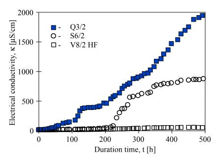
The results obtained reveal that Accurel PP V8/2 HF membranes are very resistant to pore wettability. Therefore, for the separation of salt solutions the use of thicker membranes is more advantageous.
