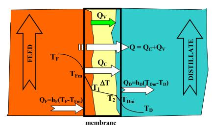
Figure 3. The heat transfer in the MD module with partially wetted membranes.
