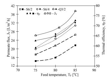
Figure 8. The influence of feed temperature and kind of used membranes on the permeate flux and thermal efficiency. Accurel PP capillary polypropylene membranes: S6/2 and V8/2 HF (0.58 cm–Table 1). Feed–distilled water.  $T_D = 20$  °C,  $m_F = m_D = 0.014$  dm<sup>3</sup>/s.
