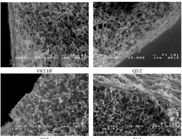
Figure 5. SEM images of cross section of Accurel PP membranes.
