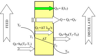
The thermal conductivity coefficient ( $\lambda_m$ ) for membranes utilized in the MD changes is in a small range: 0.04–0.06 W/mK, and can be determined on the basis of the membrane material data [1]:
