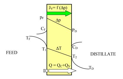
According to Equation 1 the permeate flux increases along with an increase in the membrane porosity and pore diameter, and when the membrane wall thickness is reduced. However, the thin membranes can undergo mechanical damage and become wet more easily [6,9,12]. In MD process
