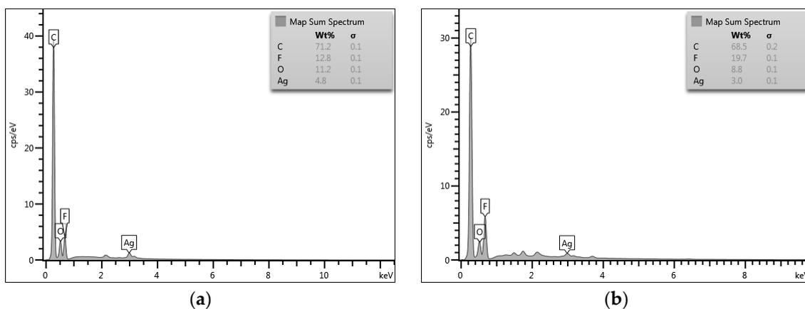
**Figure 2.** Energy dispersive X-ray (EDX) data of (a) Ag/PVDF-HFP and (b) Ag-MWCNTs/PVDF-HFP.
