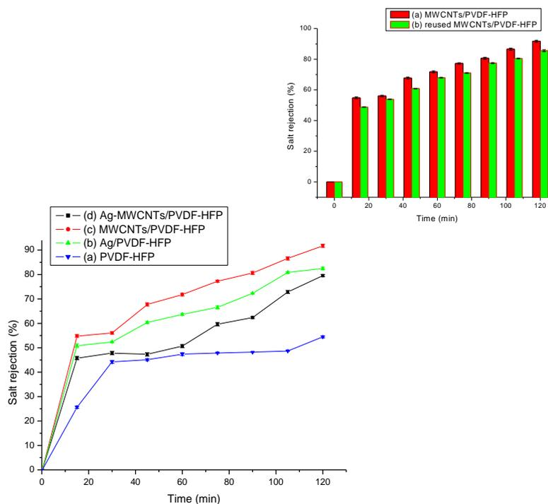
**Figure 8.** Salt rejection tests of the permeate solution after filtration using (a) PVDF-HFP, (b) Ag/PVDF-HFP, (c) MWCNTs/PVDF-HFP (d) Ag-MWCNTs/PVDF-HFP membrane and the insert showing the 1st and 3rd filtration cycles of salt rejection using MWCNTs/PVDF-HFP membrane.
