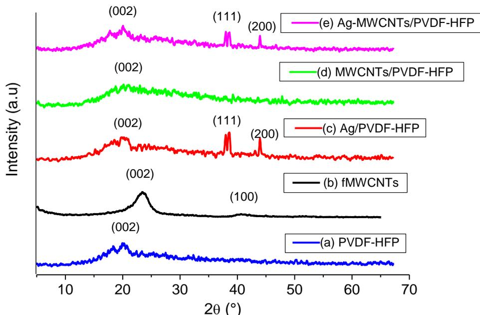
**Figure 1.** X-ray diffraction patterns of (a) poly(vinylidene fluoride-co-hexafluoropropene) (PVDF-HFP), (b) fMWCNTs, (c) Ag/PVDF-HFP, (d) MWCNTs/PVDF-HFP, (e) Ag-MWCNTs/PVDF-HFP.
