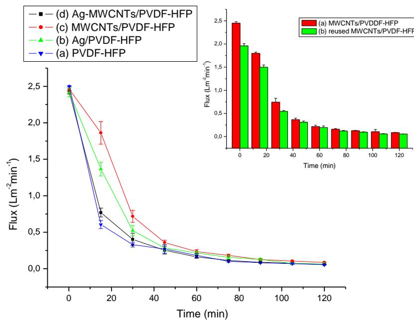
**Figure 7.** Filtrate flux for salted water (2000 ppm) filtered through the (a) PVDF-HFP, (b) Ag/PVDF-HFP, (c) MWCNTs/PVDF-HFP, and (d) Ag-MWCNTs/PVDF-HFP membranes, and the insert showing the 1st and 3rd filtration cycles of filtrate flux for MWCNTs/PVDF-HFP membrane.
