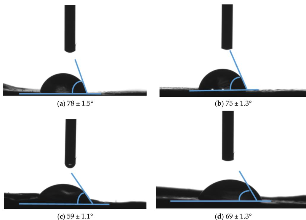
**Figure 6.** Contact angle measurements of (a) PVDF-HFP; (b) Ag/PVDF-HFP, (c) MWCNTs/PVDF-HFP and (d) Ag-MWCNTs/PVDF-HFP.
