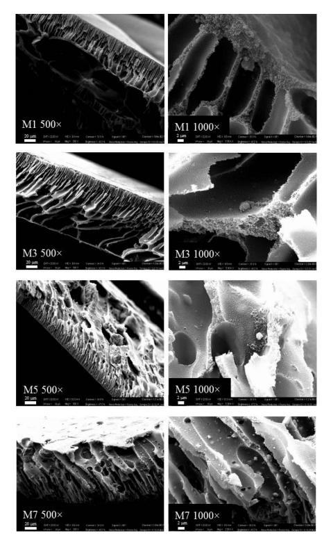
**Figure 2.** Scanning electron microscopy (SEM) images of the PES and PES–kaolin membranes prepared via the Non-solvent Induced Phase Separation (NIPS) procedure.
