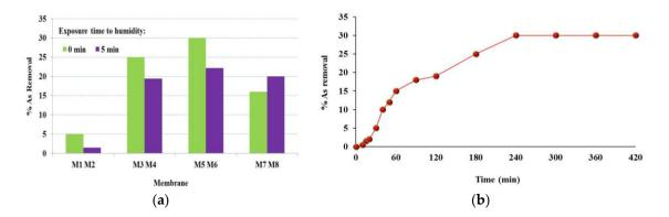
**Figure 5.** (a) As adsorption after 240 min test by using PES and PES–kaolin membranes prepared via NIPS and NIPS–VIPS; (b) Kinetic of As adsorption on the M5 PES–kaolin membrane.
