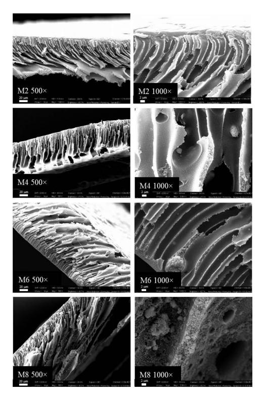
**Figure 3.** SEM images of the PES and PES–kaolin membranes prepared via NIPS–Vapour Induced Phase Separation (VIPS) procedure.
