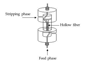
**Figure 1.** Scheme of the module used in the hollow fibre supported liquid membrane (HFSLM) experiments.
