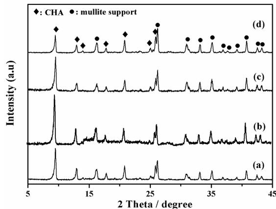
**Figure 4.** XRD patterns of high silica SSZ-13 zeolite membranes with different  $H_2O/SiO_2$  ratio, (a) M-4,  $H_2O/SiO_2 = 20$ ; (b) M-5,  $H_2O/SiO_2 = 40$ ; (c) M-6,  $H_2O/SiO_2 = 60$ ; (d,b) M-3,  $H_2O/SiO_2 = 80$ .
