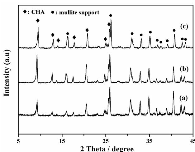
**Figure 2.** XRD patterns of high silica SSZ-13 zeolite membranes with different  $\text{SiO}_2/\text{Al}_2\text{O}_3$  ratio; (a) M-1,  $\text{SiO}_2/\text{Al}_2\text{O}_3 = 40$ ; (b) M-2,  $\text{SiO}_2/\text{Al}_2\text{O}_3 = 200$ ; (c) M-3,  $\text{SiO}_2/\text{Al}_2\text{O}_3 = \infty$ .
