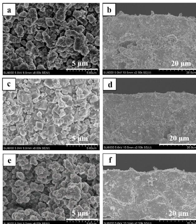
**Figure 3.** Surface and cross-sectional SEM images of high silica SSZ-13 zeolite membranes with different  $\text{SiO}_2/\text{Al}_2\text{O}_3$  ratio (a,b) M-1,  $\text{SiO}_2/\text{Al}_2\text{O}_3 = 40$ ; (c,d) M-2,  $\text{SiO}_2/\text{Al}_2\text{O}_3 = 200$ ; (e,f) M-3,  $\text{SiO}_2/\text{Al}_2\text{O}_3 = \infty$ .
