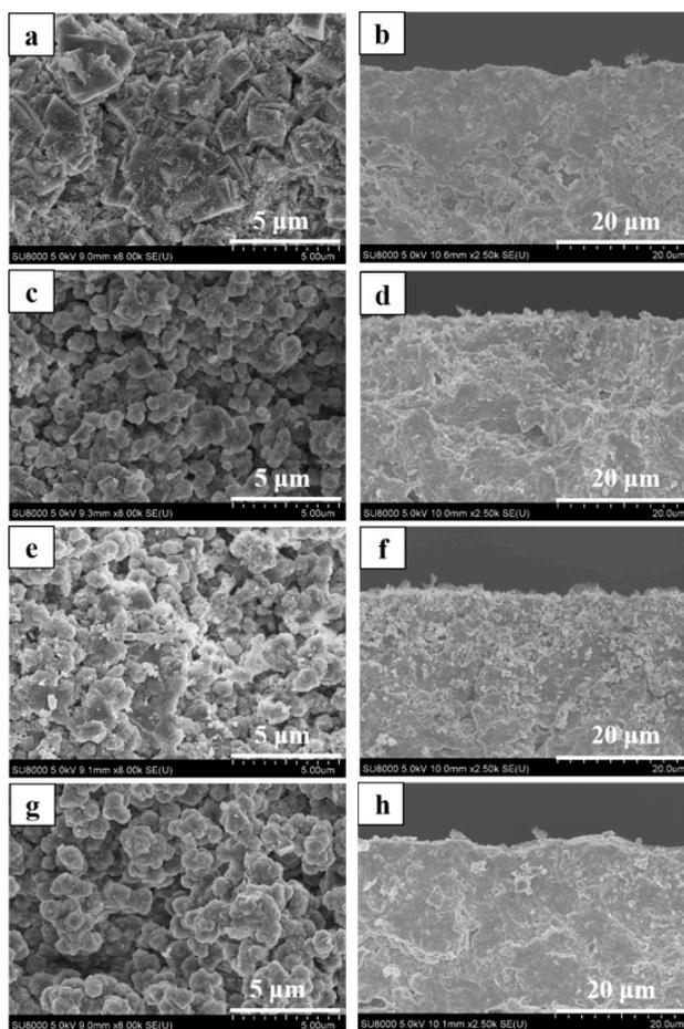
**Figure 5.** Surface and cross-sectional SEM images of high silica SSZ-13 zeolite membranes with different  $H_2O/SiO_2$  ratio, (a,b) M-4,  $H_2O/SiO_2 = 20$ ; (c,d) M-5,  $H_2O/SiO_2 = 40$ ; (e,f) M-6,  $H_2O/SiO_2 = 60$ ; (g,h) M-3,  $H_2O/SiO_2 = 80$ .
