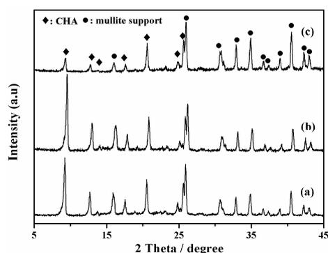
**Figure 6.** XRD patterns of high silica SSZ-13 zeolite membranes with different TMAdaOH/SiO<sub>2</sub> ratio, (a) M-7, TMAdaOH/SiO<sub>2</sub> = 0.05; (b) M-4, TMAdaOH/SiO<sub>2</sub> = 0.10; (c) M-8, TMAdaOH/SiO<sub>2</sub> = 0.15.
