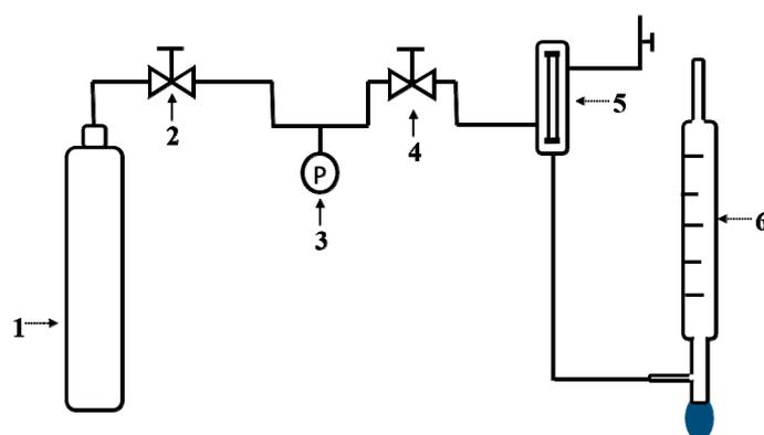
**Figure 1.** Single gas permeation measurements: (1) cylinder; (2) reducing valve; (3) pressure gauge; (4) counterbalance valve; (5) membrane module; (6) soap bubble flowmeter.
