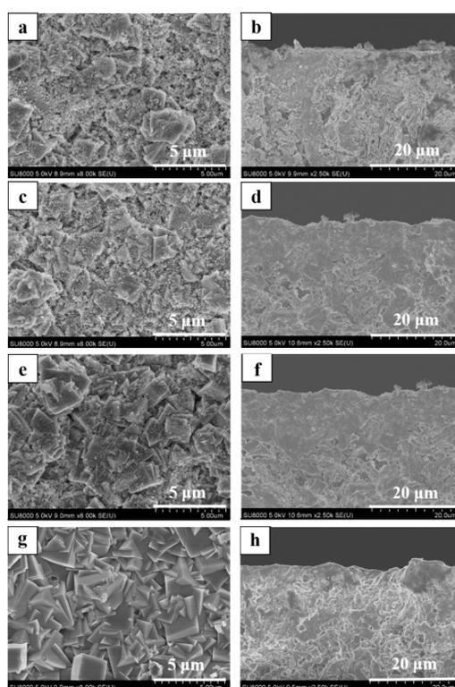
**Figure 9.** Surface and cross-sectional SEM images of high silica SSZ-13 zeolite membrane with different synthesis time, (a,b) M-9, 24 h; (c,d) M-10, 36 h; (e,f) M-4, 48 h; (g,h) M-11, 72 h.
