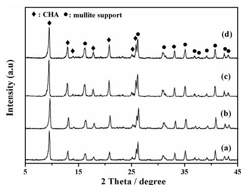
**Figure 8.** XRD patterns of high silica SSZ-13 zeolite membrane with different synthesis time, (a) M-9, 24 h; (b) M-10, 36 h; (c) M-4, 48 h; (d) M-11, 72 h.
