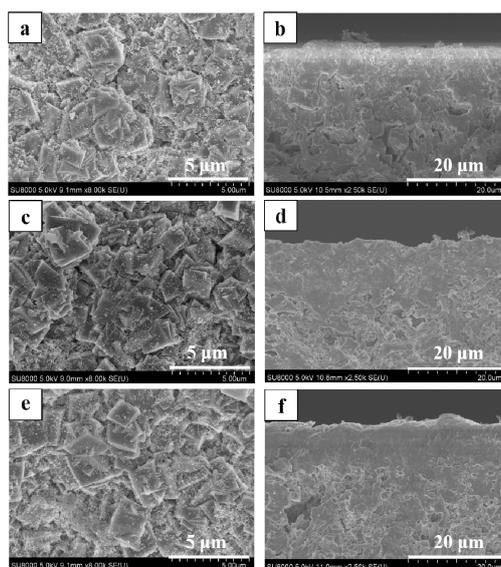
**Figure 7.** Surface and cross-sectional SEM images of high silica SSZ-13 zeolite membranes with different TMAdaOH/SiO<sub>2</sub> ratio, (a,b) M-7, TMAdaOH/SiO<sub>2</sub> = 0.05; (c,d) M-4, TMAdaOH/SiO<sub>2</sub> = 0.10; (g,h) M-8, TMAdaOH/SiO<sub>2</sub> = 0.15.
