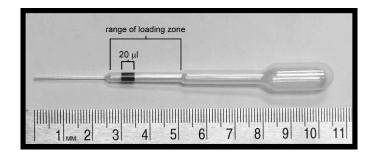
**Figure 2.** Loading of a Samco 231 disposable fine-tip pipette with HDCs. A 20 mL volume of opaque liquid has been loaded into this pipette. The numbers on the scale indicate centimeters.
