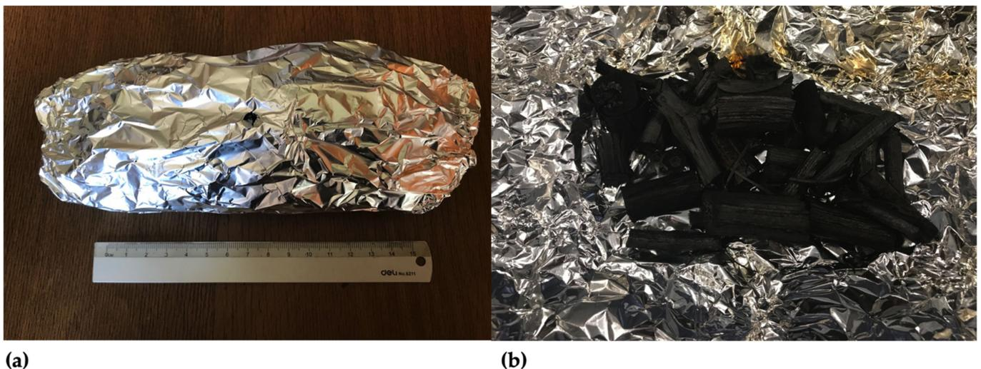
Figure 2. (a) Material wrapped in the aluminum foil; (b) produced biochar.
