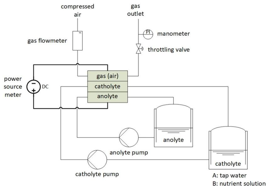
**Figure 3.** Setup for the electrochemical H<sub>2</sub>O<sub>2</sub> production with a three-compartment (gas, catholyte, and anolyte) electrolysis cell. In the ex situ production scenario, tap water (A) was used as the catholyte, and the resulting H<sub>2</sub>O<sub>2</sub> was subsequently added once to the nutrient solution. In the in situ H<sub>2</sub>O<sub>2</sub> production scenario (B), the nutrient solution was directly circulated as a catholyte through the electrolysis cell.
