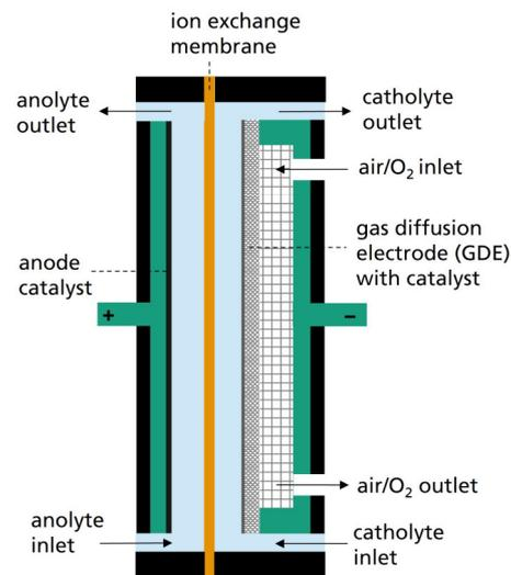
**Figure 2.** Schematic of the electrolysis cell for H<sub>2</sub>O<sub>2</sub> production on a gas diffusion electrode.
