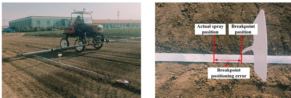
**Figure 8.** Experimental scene of breakpoint identification and positioning accuracy.
