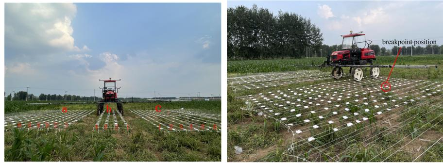
**Figure 9.** Test scene for droplet deposition measurement. Where numbers correspond to the number of columns, “abc” corresponded to the different regions.
