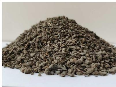
**Figure 1.** Particulate materials in residual film mixture after sieving.
